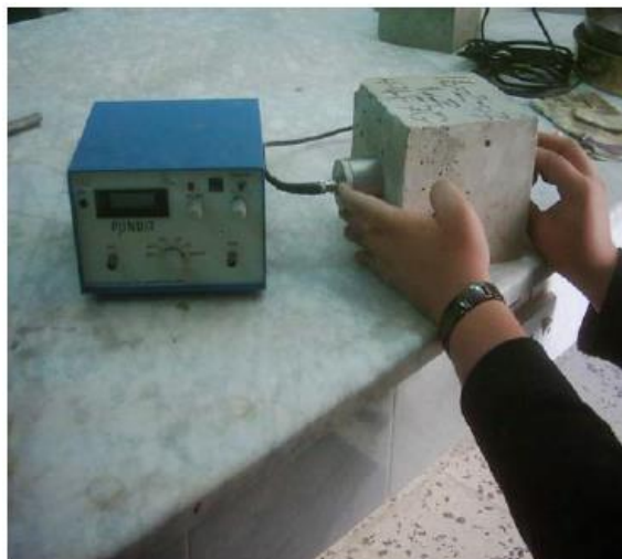
Testing using PUNDIT
