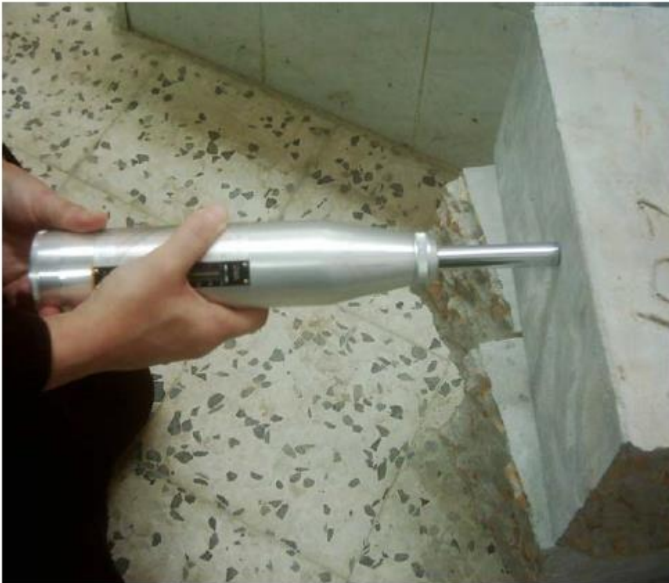
Testing concrete using the Schmidt hammer
