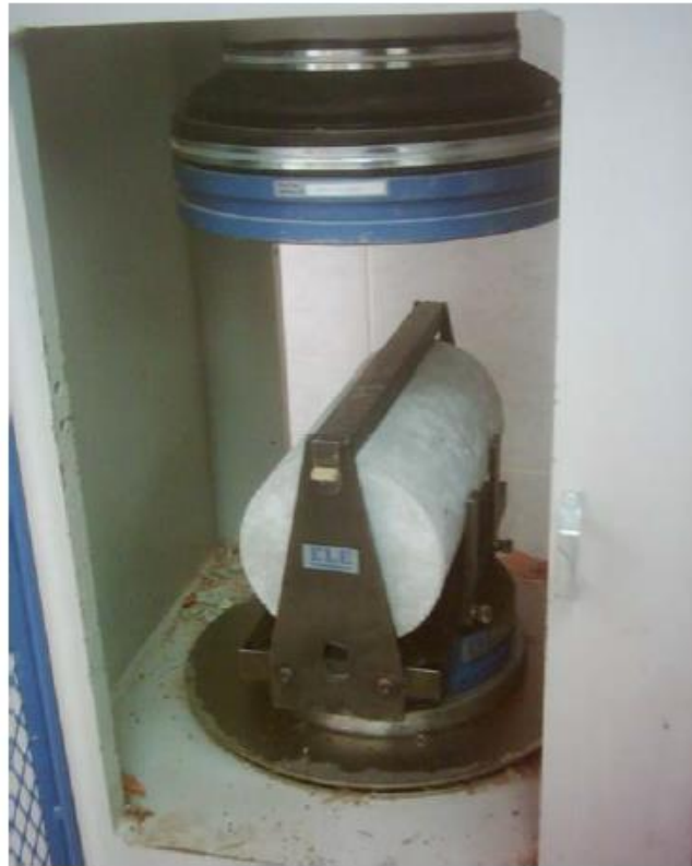
Cylinder in the compression machine with the jig for aligning concrete cylinder and bearing strips
