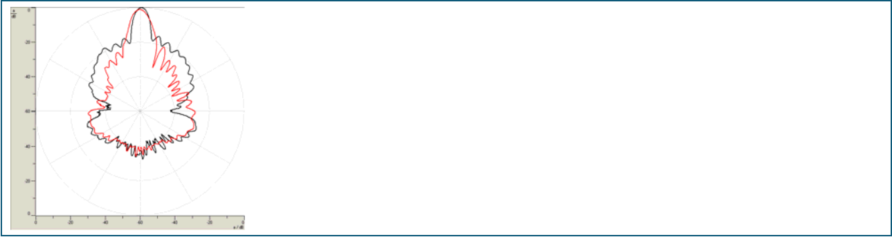
E-plane Polar coordinates Linear representation: A(\theta) Black: Excitation with \lambda/2 -dipole Red: Excitation with Yagi-DR
