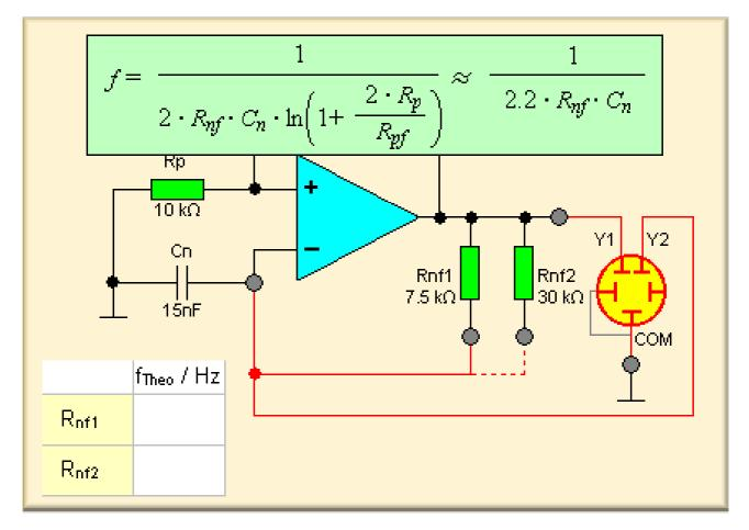
The multivibrator has a positive as well as a negative feedback. The negative feedback branch consists of the RC element  $R_{nf}$  and  $C_n$ , and the positive feedback branch of the voltage divider  $R_{pf}$  and  $R_p$ , which fixes the threshold voltages of the hysteresis. The frequency of the system depends on the voltage division ratio and the time constant of the RC element.
