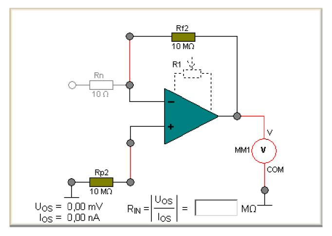
Operational amplifiers have a very high input resistance. The offset voltage is caused by the input resistance in conjunction with the input offset current. Because of the high input resistance and the low output resistance it is possible to set up an impedance transformer<sup>1</sup> with an OPA circuit.
