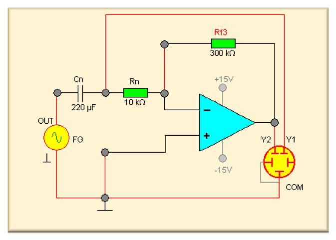
In theory, the output voltage would exceed the supply voltage in case of too great a gain or too high an input voltage. Therefore the operational amplifier cuts off the signal when it reaches the limits of the output range. The magnitude of these limits is about 1...3 V below the supply voltages. There are also OPAs with a so-called rail-to-rail<sup>1</sup> output range.
