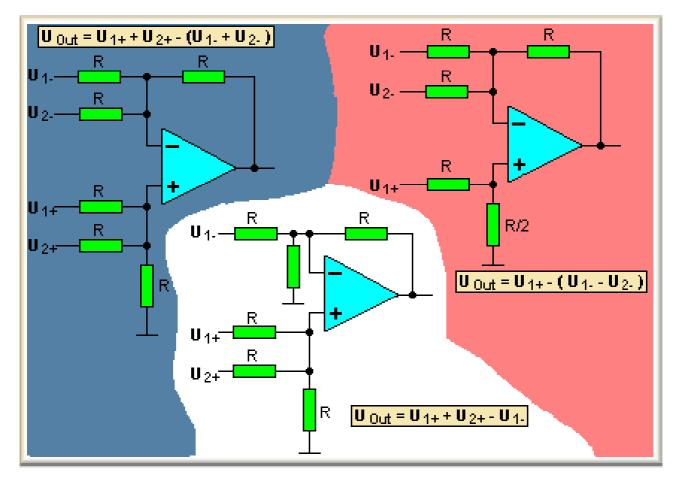
Like the adder, the subtractor can be extended.
