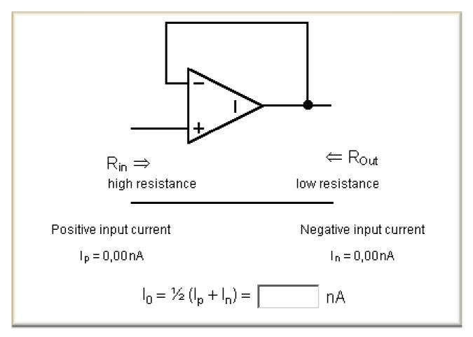
The input bias current  $I_0$  is the mean value of the positive and negative input current:
