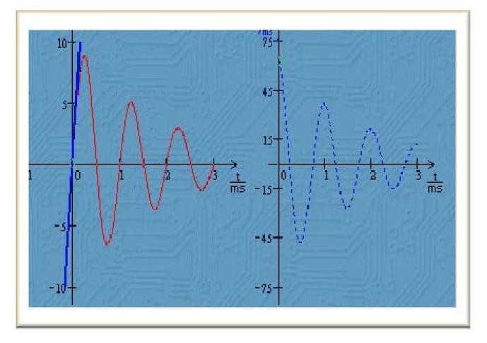
The output of a differentiator is proportional to the time derivative of a signal, which describes the time rate of change of a signal. The value corresponds to the slope of the tangent at the curve at time t.
