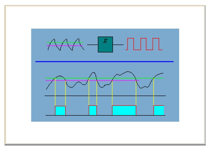
The Schmitt trigger is employed, e.g., in communications engineering in order to convert noisy digital signals into "clean" rectangular signals. Schmitt triggers are, among other things, also contained in the serial interfaces of a computer.
