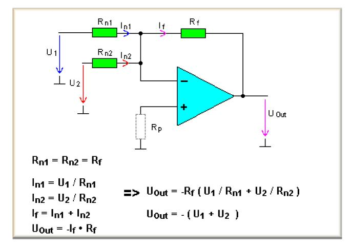
The example shows how the addition of two voltages is realised. Because the inverting input is Virtually grounded (neglect of the voltage drop at  $R_P$ ), the summer can be arbitrarily extended.
