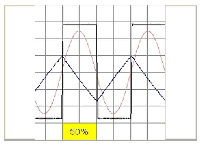
In the animation the signals are shown altogether. The percentage given is the duty cycle<sup>1</sup> of the rectangular function. A symmetric rectangular signal would be free of d.c. components for a duty cycle of 50 %
