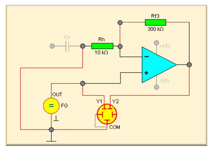
The output voltage and input voltage at a non-inverting amplifier have equal signs (for d.c. and low frequencies). So the a.c. signal at the output is in phase with the input signal.
