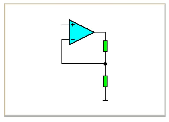
In the case of a non-inverting operational amplifier the signal to be amplified is fed into the non-inverting input. Therefore the signs of the output voltage and the input voltage are equal. However, the feedback takes place via the inverting input as in the case of the inverting amplifier. The input signal is loaded with a very small positive input current. So the control is powerless<sup>1</sup>.
