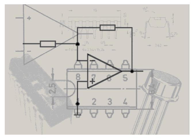
The inverting amplifier is used in communications, measuring and control engineering. Moreover, it is the basis of many applications, some of which are described in the following chapters, e.g. integrators, differentiators and active filter circuits.
