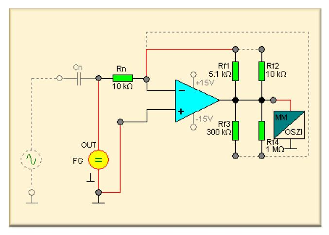
In this last experiment of this chapter another fault has been activated. Check **all** kinds of circuits of the inverting amplifier one after another and try to track down the fault. Use the multimeters or the oscilloscope for your measurements. Vary the input signal (supply d.c. after  $C_n$ , a.c. before  $C_n$ ).
