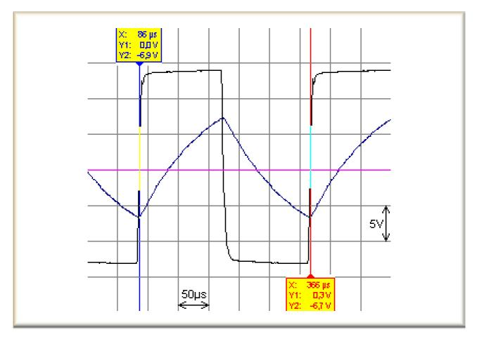
The output signal is a rectangular function. The potential at the inverting input corresponds to the charging and discharging curve of an RC element.
