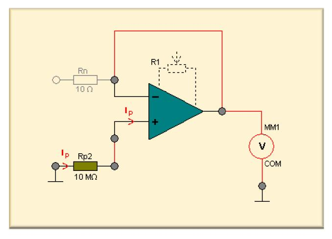
The positive input current is the current that flows through the non-inverting input. It cannot be measured directly because it is in of the order of magnitude of nA. There is a voltage drop at  $R_{p2}$  due to the input current. The gain is 1 because there are no resistances in the feedback. We have  $U_{out} = -U_{rp2}$ . The positive input current therefore is:
