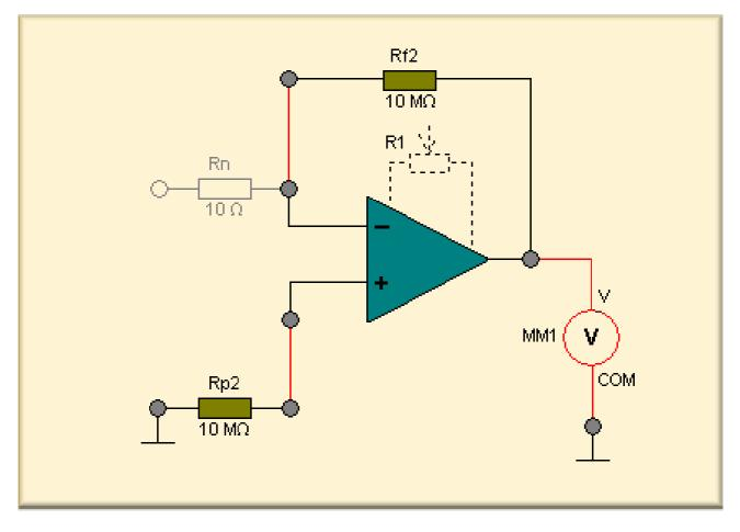
The input offset current  $I_{OC}$  is the difference between the positive and the negative input current. The offset voltage is caused by the input current in conjunction with the input resistance.
