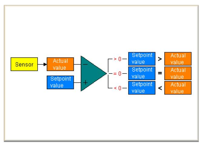
Comparators are used, e.g., for comparing a signal with a setpoint value. If the signal deviates from the setpoint value, the output voltage is positive or negative depending on the external circuit elements and the deviation. The output voltage is changed even by the slightest deviations. In the picture the ideal case is shown, the offset not being taken into account.
