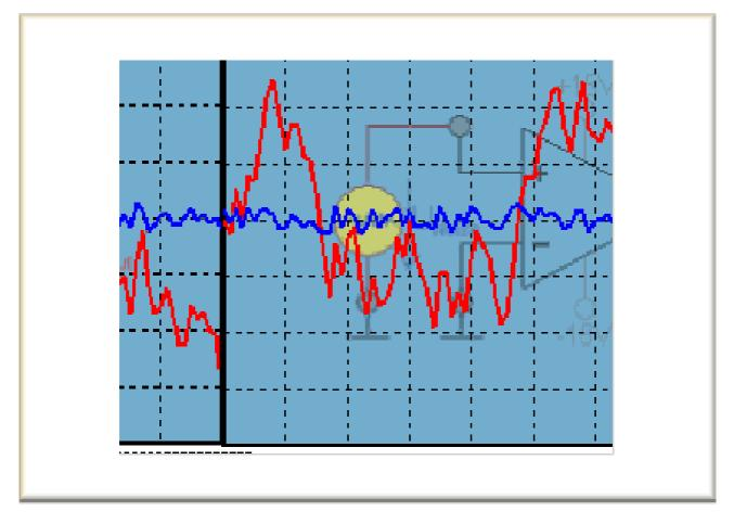
The comparator has a vital disadvantage: If the input signals are noisy, the state of the output changes several times near the switching point.
