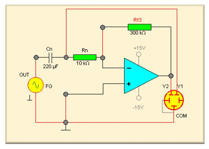
The input and output voltages of an inverting amplifier have exactly opposite signs (for d.c. and low frequencies). Thus there is a phase shift of 180° between the output and the input signal.
