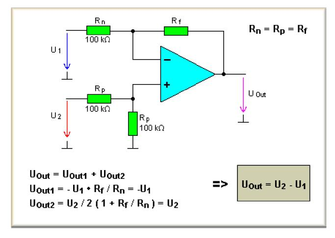
The signal to be subtracted is fed into the inverting input. This causes a difference voltage, to which the output voltage is proportional.
