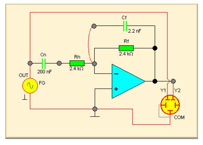
The bandpass filter is a combination of a high-pass and a low-pass filter. Its transfer function corresponds to the product of the two individual transfer functions.
