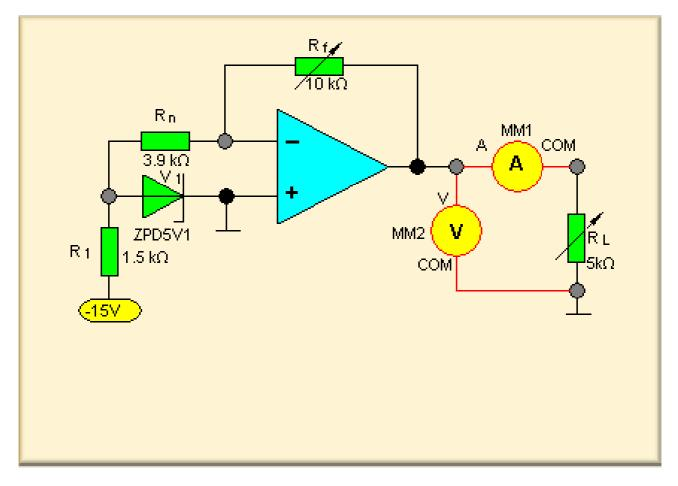
A negative voltage stabilised by a Zener diode is applied to the inverting branch and causes a constant positive output voltage, which can be adjusted via the gain ( $R_f / R_n$ ).
