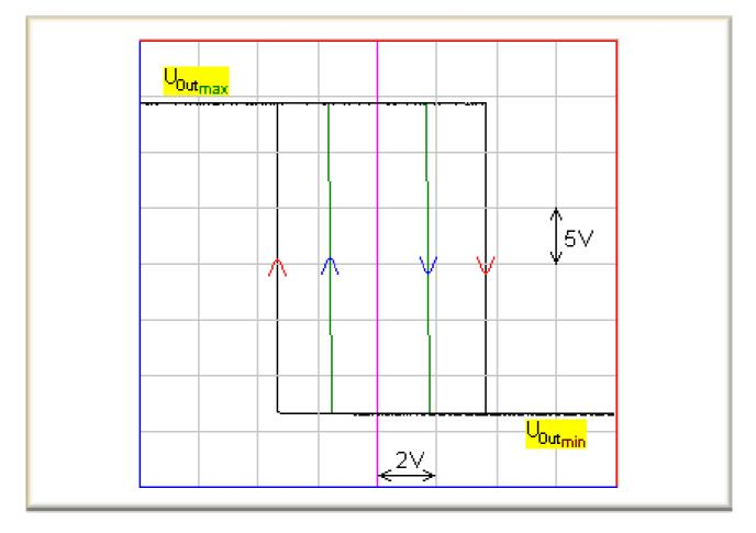
The hysteresis values do not depend on the resistances alone, but also on the limits of the OPA's dynamic range. Therefore a slightly asymmetric hysteresis results because the negative limit is usually smaller than the positive one by 1 V.
