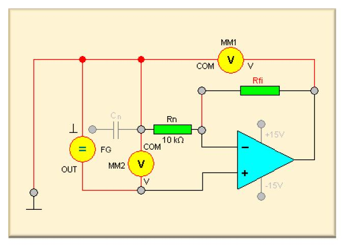
Because of the very small difference voltage between the two inputs, the inputs are approximately on the same potential. That means the voltage drop at  $R_n$  corresponds to the input voltage and the voltage drop at  $R_n$  and  $R_{fi}$  corresponds to the output voltage. Here  $R_n$  and  $R_{fi}$  form a voltage divider. The gain therefore is:
