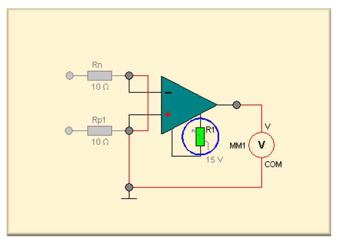
Many ICs of operational amplifiers have connections for compensating the offset by external elements. In EF1 the offset can be compensated with the resistor  $R_1$ .
