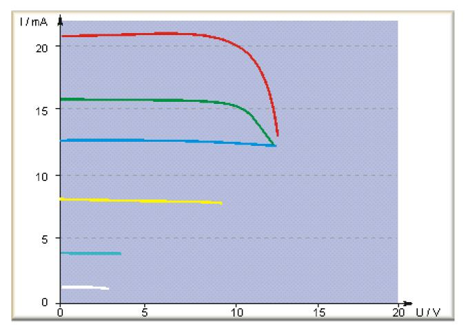
The load current remains constant until the voltage limit of the OPA is reached ( $-12 \dots -13 V$ ). After that the load current collapses.
