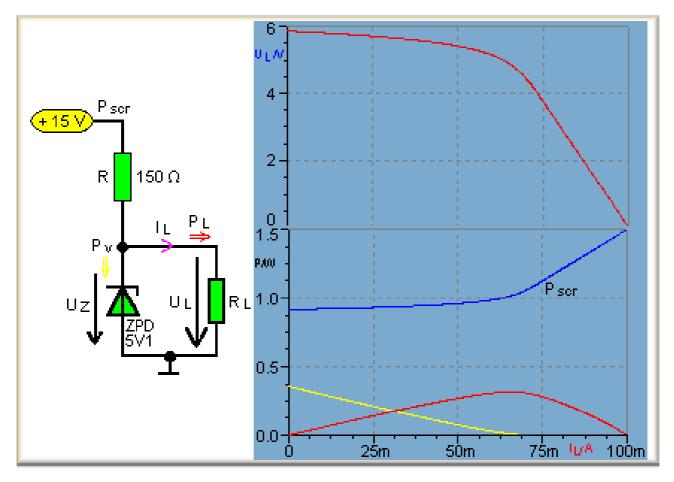
The opposite circuit is a simple constant-voltage source. The disadvantages of this circuit are the high power dissipation and a non-adjustable output voltage.
