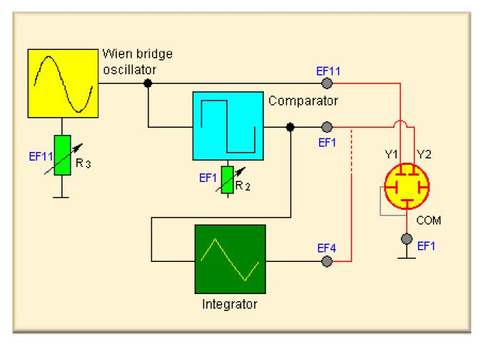
In our case, the frequency determining element is a Wien bridge (adjustment with  $R_3$  in EF11). With the comparator a rectangular signal is generated from the sinusoidal signal. The duty cycle of the rectangular signal is adjusted with  $R_2$  in EF1.
