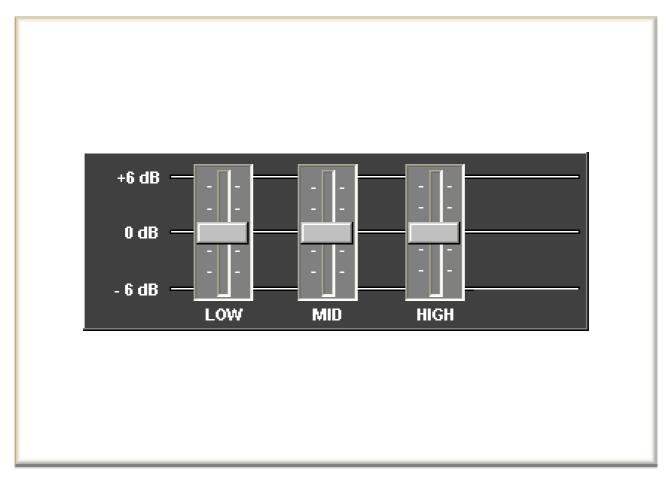
Filter circuits are often used in sound engineering for controlling sounds. With a so-called equalizer frequency ranges can be damped or amplified (highlighted).
