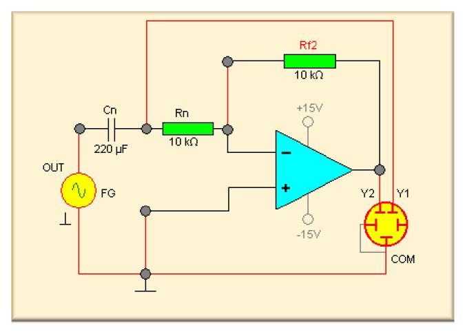
The internal capacitances and the switching times of the transistors integrated in the operational amplifier cause a change to the phase shift between the input and the output signal as the frequency increases. Please read the additional information on measuring the phase response<sup>1</sup>.
