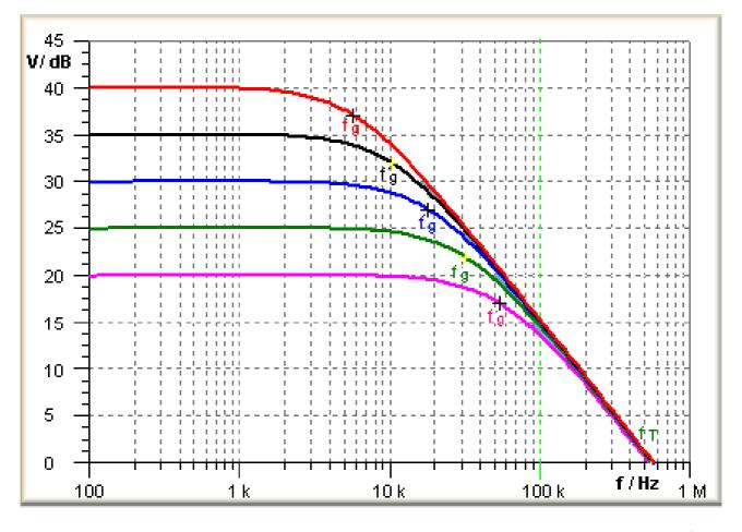
The gain-bandwidth product of an operational amplifier is constant and equal to the transition frequency<sup>1</sup>.
