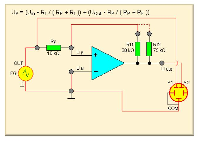
The potential  $U_{\rm p}$  can be calculated according to the principle of superposition. Here  $R_{\rm p}$  and  $R_{\rm fi}$  form a voltage divider.
