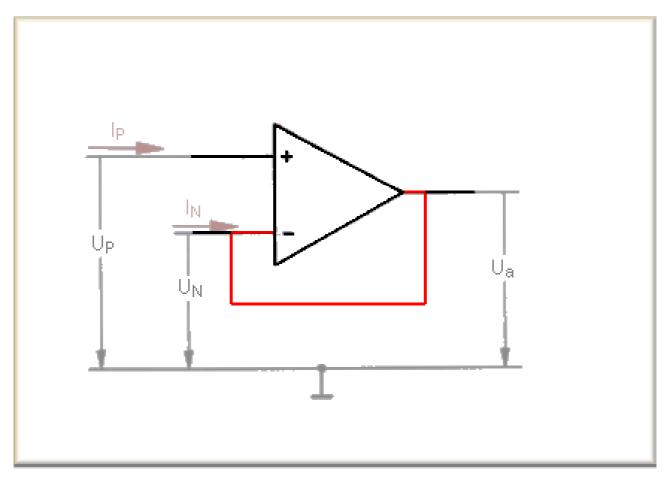
By negative feedback part of the output voltage is led back to the inverting input. This leads to a damping of the gain.
