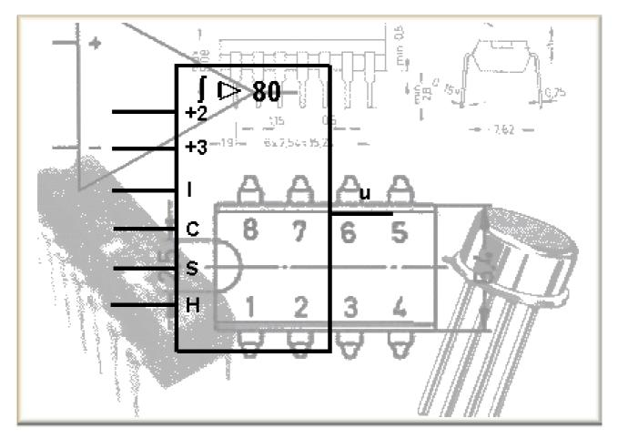
The integrator used to be employed in arithmetical circuits. Today it is of great importance in control engineering (integral-action controllers: I element<sup>1</sup>) and in designing function generators (signal shaping: rectangular to delta). Furthermore the integrator is employed, e.g., for the offset compensation in measuring amplifiers<sup>2</sup>.
