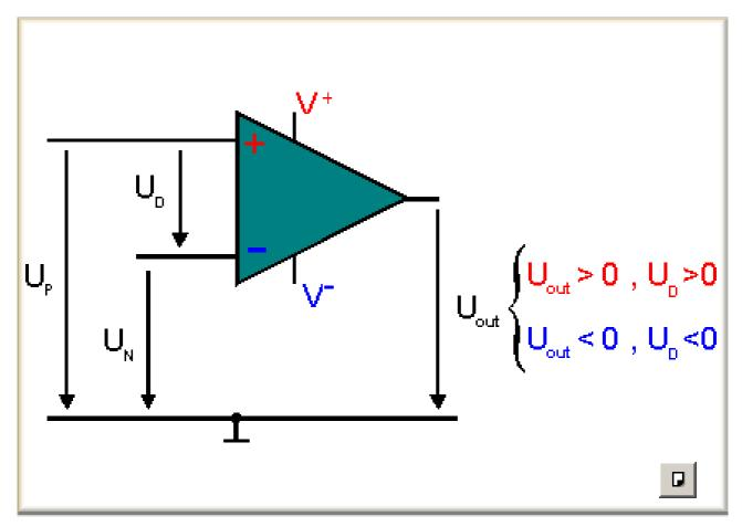
The operational amplifier has a difference amplifier<sup>1</sup> in its input. If the potential of the inverting input is higher, the output voltage is negative. If the potential of the non- inverting input is higher, the output voltage is positive. The magnitude of the output voltage depends on the difference between the input voltages and on the gain. Because of the high open-loop gain<sup>2</sup> the output is completely saturated even if the differences are small.
