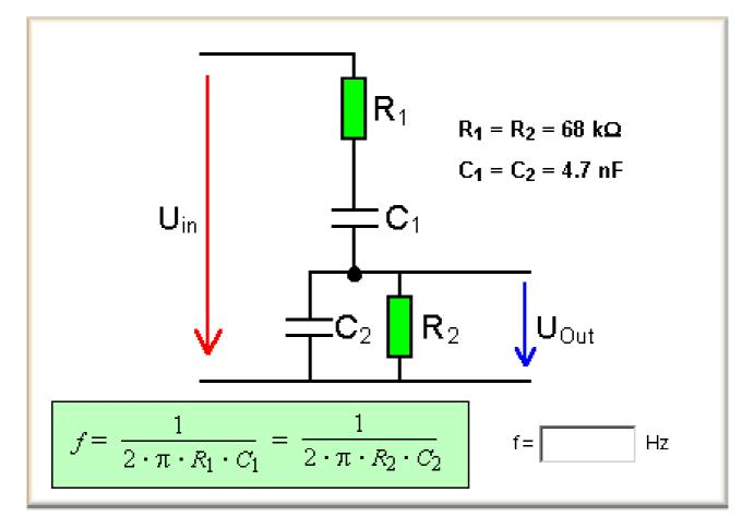
In the Wien bridge oscillator the Wien bridge is used as a frequency dependent voltage divider. At the frequency determined by the RC elements the output voltage  $U_{out}$  of the Wien bridge has its maximum value and the phase difference between  $U_{out}$  and  $U_{In}$  is 0°.
