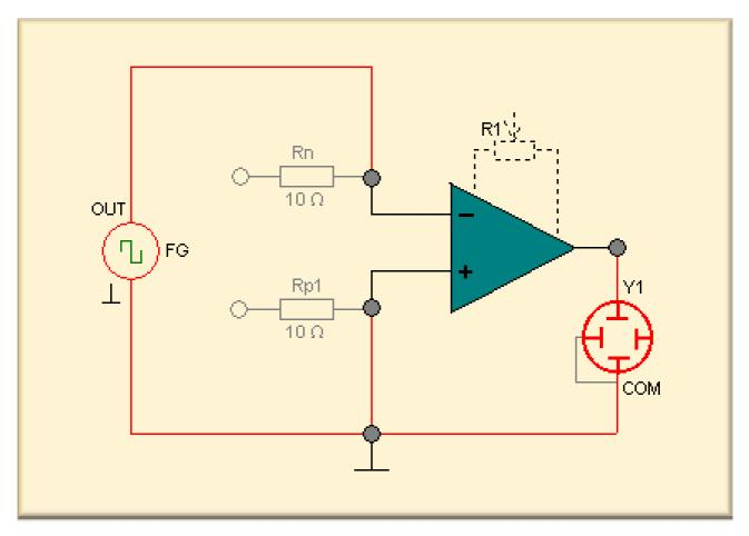
If the input signal at the OPA changes as a function of time, the output signal will follow it. However, due to internal capacitances this response cannot take place at an arbitrary rate. The slew rate (SR) is the maximum steepness of the leading edge of the output voltage. It is a measure for the switching speed of an operational amplifier. Its is given in units of  $V/\mu s$ .
