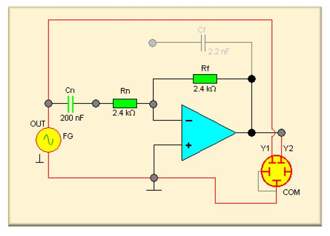
The circuit consists of an inverting amplifier with a frequency dependent input impedance ( $R_n$  and  $C_n$ ). The impedance of  $C_n$  is high for low frequencies and becomes lower and lower as the frequency increases.
