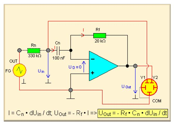
In the case of the differentiator, the charging voltage of the capacitor is the input voltage. The output voltage is the voltage generated by the charging current of the capacitor at  $R_{\rm f}$ .
