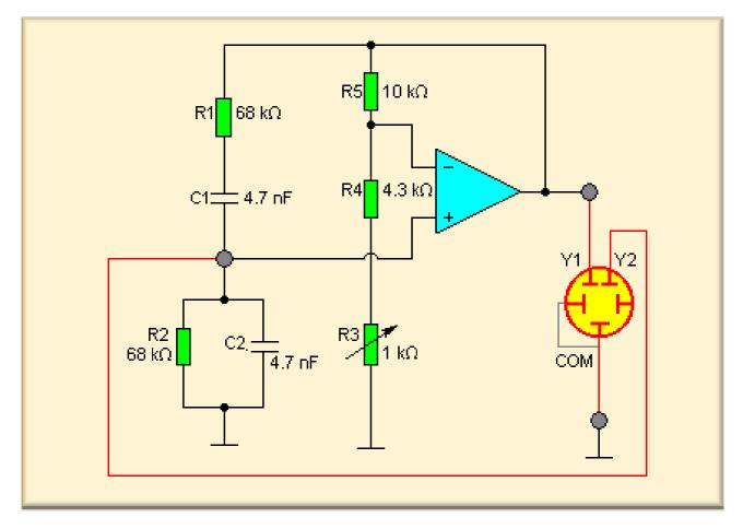
The RC elements ( $R_1$ ,  $C_1$  and  $R_2$ ,  $C_2$ ) of the Wien bridge determine the positive feedback and thus the frequency of the oscillation.  $R_3$ ,  $R_4$  and  $R_5$  form a voltage divider. They determine the negative feedback and thus the course (the amplitude) of the oscillation. If the negative feedback is too strong, the oscillation stops. If the negative feedback is too weak, the positive feedback predominates and the OPA is overloaded.
