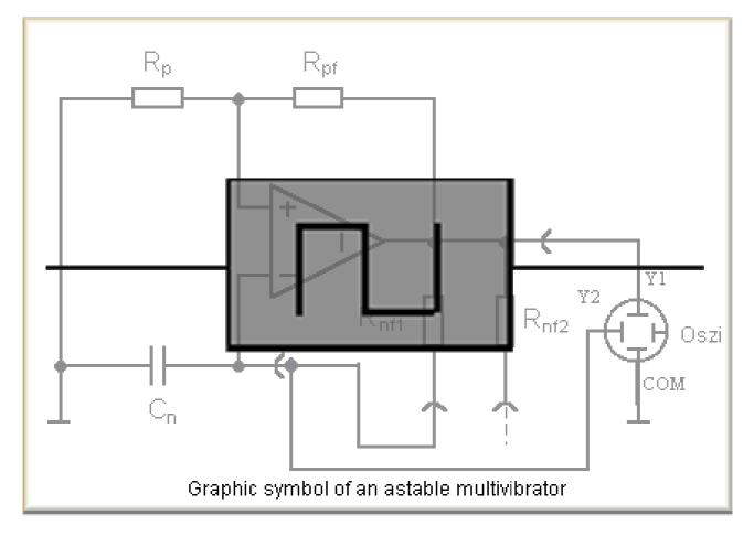
The astable multivibrator generates a rectangular signal with constant amplitude and frequency without external excitation. That means it is an oscillating circuit.
