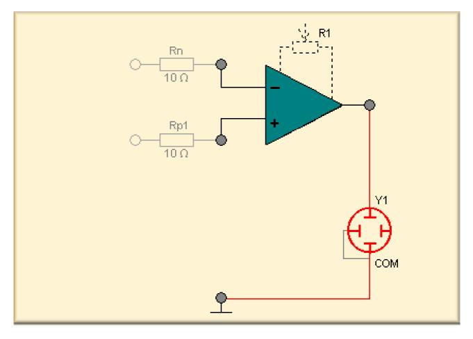
In the case of a difference amplifier, only the difference between the two input signals is relevant. Components that are equal in both signals (common mode) cancel in the difference and are thus suppressed by the difference amplifier.
