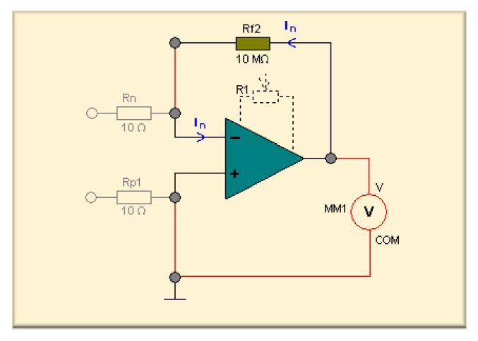
The negative input current is the current that flows through the inverting input. In cannot be measured directly because it is of the order of magnitude of nA. There is a voltage drop at  $R_{f2}$  due to the input current. As the inverting input is Virtually grounded ( $U_D = 0$ ), we have  $U_{out} = +U_{rf2}$ . The negative input current therefore is:
