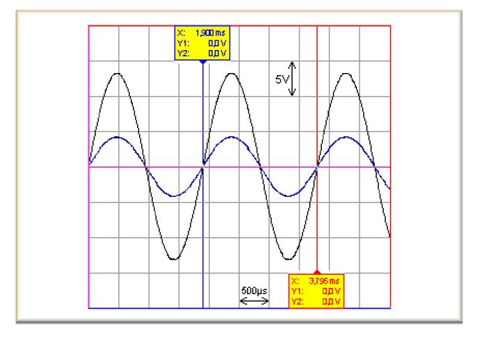
The frequency of the signal is approximately 500 Hz.
