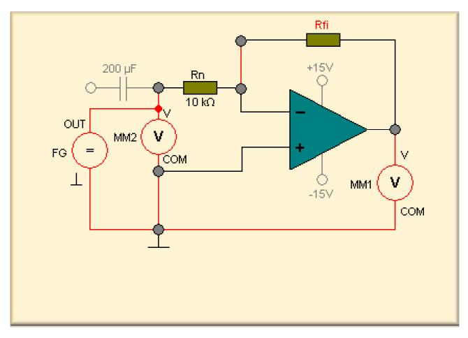
The gain is the ratio of the output voltage and the input voltage:
