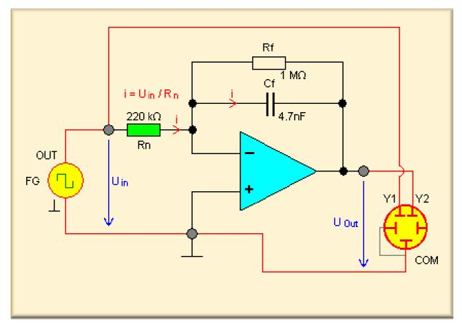
The output voltage is the charging voltage of the capacitor. The charging current is determined by  $R_n$  and by the input voltage. From this
