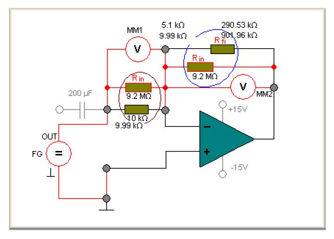
According to the theory the gains should be equal in both experiments. For higher gains this is not the case here because of the internal resistance of the multimeter (real multimeters<sup>1</sup>). The internal resistance of the multimeter is connected in parallel to the feedback resistance  $R_{fi}$ , which results in a reduction of the feedback resistance and of the gain.
