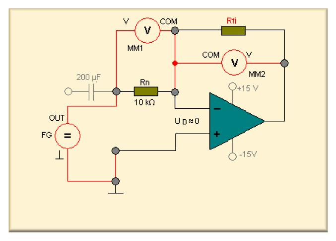
Because of the low difference input voltage the inverting input is almost grounded. That means the voltage drop at  $R_n$  corresponds to the input voltage and the voltage drop at  $R_{f1}$  to the output voltage. The gain therefore is:
