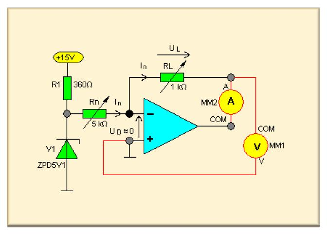
As the load resistor  $R_L$  is in the feedback branch, the output voltage is readjusted when the load changes. The current generated by the output voltage and the load resistor is therefore constant. It is equal to the current adjusted via the Zener voltage and  $R_n$ .
