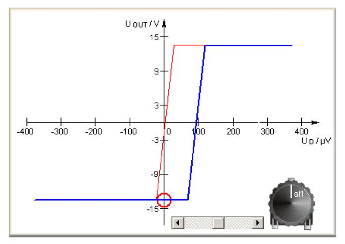
There is a position where the polarity of the output voltage changes either from positive to negative values or vice versa.
