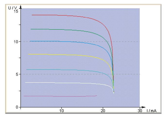
The output voltage (U < 12 V) remains stable until a maximum current (typically approx. 25 mA for the OPA) is exceeded. After that the voltage collapses.
