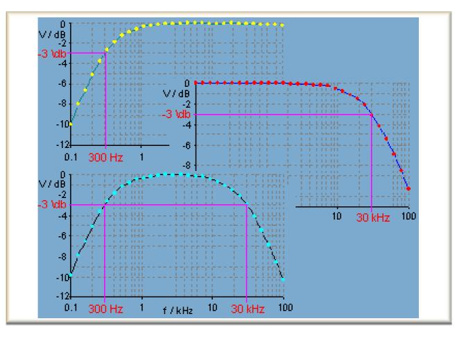
The cutoff frequency of the high-pass filter (HP) is approximately 300 Hz (245 ... 385 Hz)
