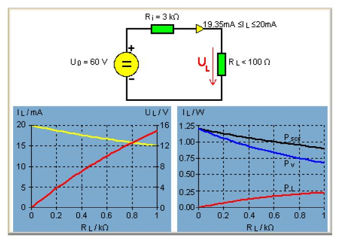
A simple constant-current source can be realised, e.g., by series connection of a high-ohmic resistor  $R_i$  and a voltage source  $U_0$ . If the short-circuit current shall not be minute, the voltage  $U_0$  has to be very high. Moreover, the load resistance has to be considerably smaller than  $R_i$ . Another disadvantage is the high power dissipation ( $P_D$ ) in the series resistor  $R_i$ .
