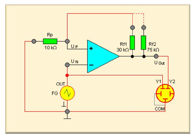
The positive feedback leads part of the output voltage  $U_{out}$  back to the non-inverting input ( $U_P$ ). Therefore the input voltage at the inverting input ( $U_N$ ) has to exceed or fall below a certain value in order that the sign of the output voltage changes. The following switching conditions are obtained:
