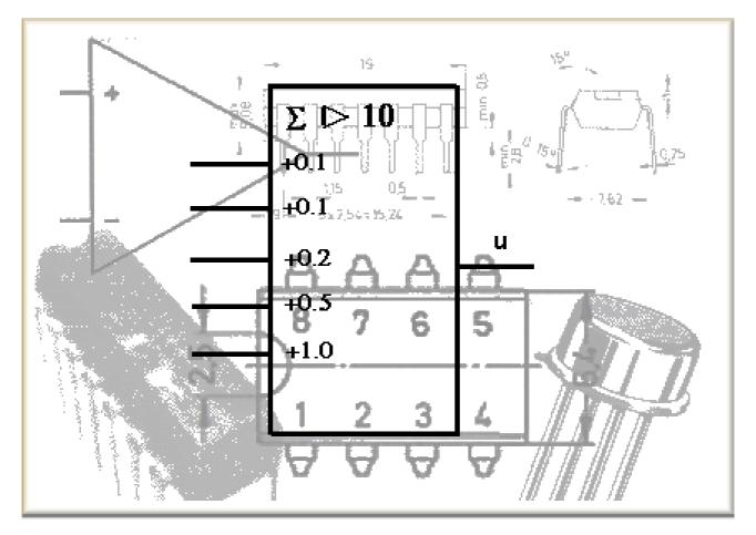
It is easy to extend the inverting amplifier so that it forms a summer. Several input resistances of equal magnitude allow an arbitrary number of voltages to be added. The negative output voltage is then proportional to the sum of the input voltages.
