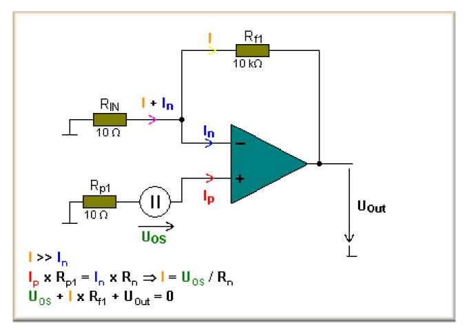
The offset voltage<sup>1</sup> is the input difference voltage at which the output voltage is 0 V.
