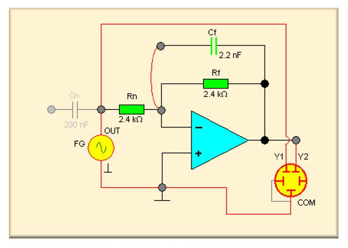
The circuit consists of an inverting amplifier (d.c. gain of -1) with a frequency dependent feedback impedance (R<sub>f</sub> and C<sub>f</sub>). The impedance of C<sub>f</sub> and thereby the feedback impedance decreases with increasing frequency.
