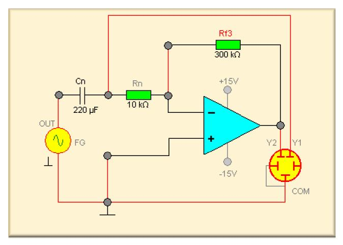
Internal capacitances lead to a reduction of the gain with increasing frequency. At the cutoff frequency<sup>1</sup> the gain of the OPA has fallen by a factor of  $1/\sqrt{2} \approx 0.707$  (= 3dB) compared with its maximum value. Without frequency dependent external circuit elements, the OPA has its maximum gain in the case of direct voltage.
