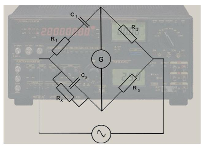
Wien bridge oscillators are employed in analog function generators for generating low-frequency sinusoidal signals. They belong to the RC oscillators and are used in the frequency range from 0.1 Hz up to about 100 Hz.
