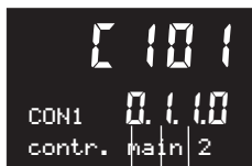
Main controller configuration 2:
