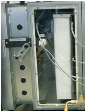
Fig. 2.7 Air filter and louvered flaps to front left
