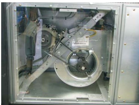
Fig. 2.13 Fan with belt drive in ET 620
