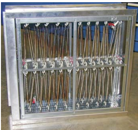
Fig. 2.10 Air heater when removed
