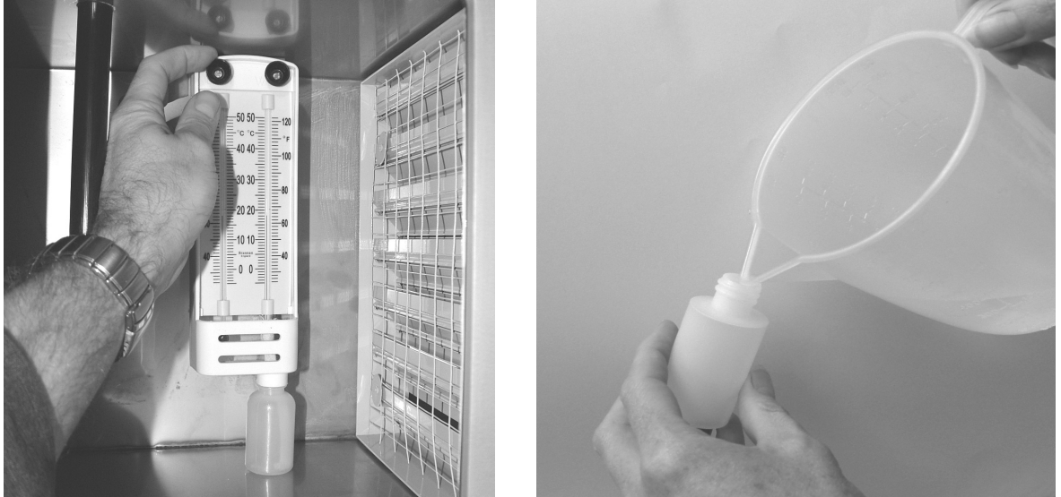
Figure 11 Unscrew the Wet and Dry Hygrometer, then Fill its Bulb with Cold Water
