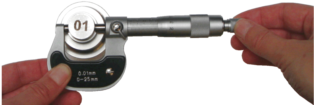
Fig. 4.12 Measuring a diameter with the micrometer 0...25 mm
