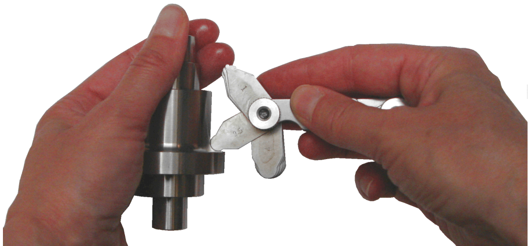
Fig. 4.13 Gauging a radius with the convex radius gauge
