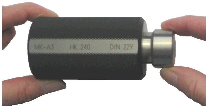
Fig. 4.13 Testing the angle and shape of an external taper
