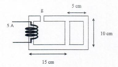
The magnetic circuit shown has  $\mu_r = 20000$ . Find the percentage increase in the total flux if the gap length decreases from 2 mm to 1 mm
