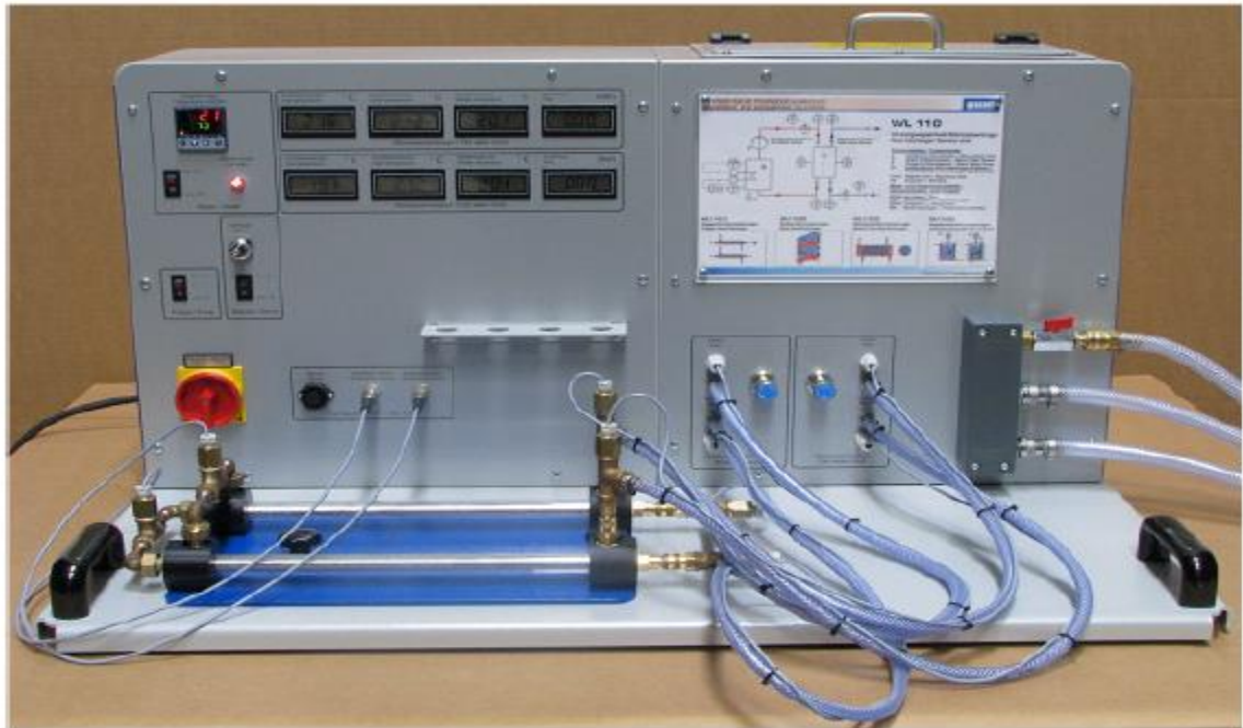
Fig 5: Tubular heat exchanger
