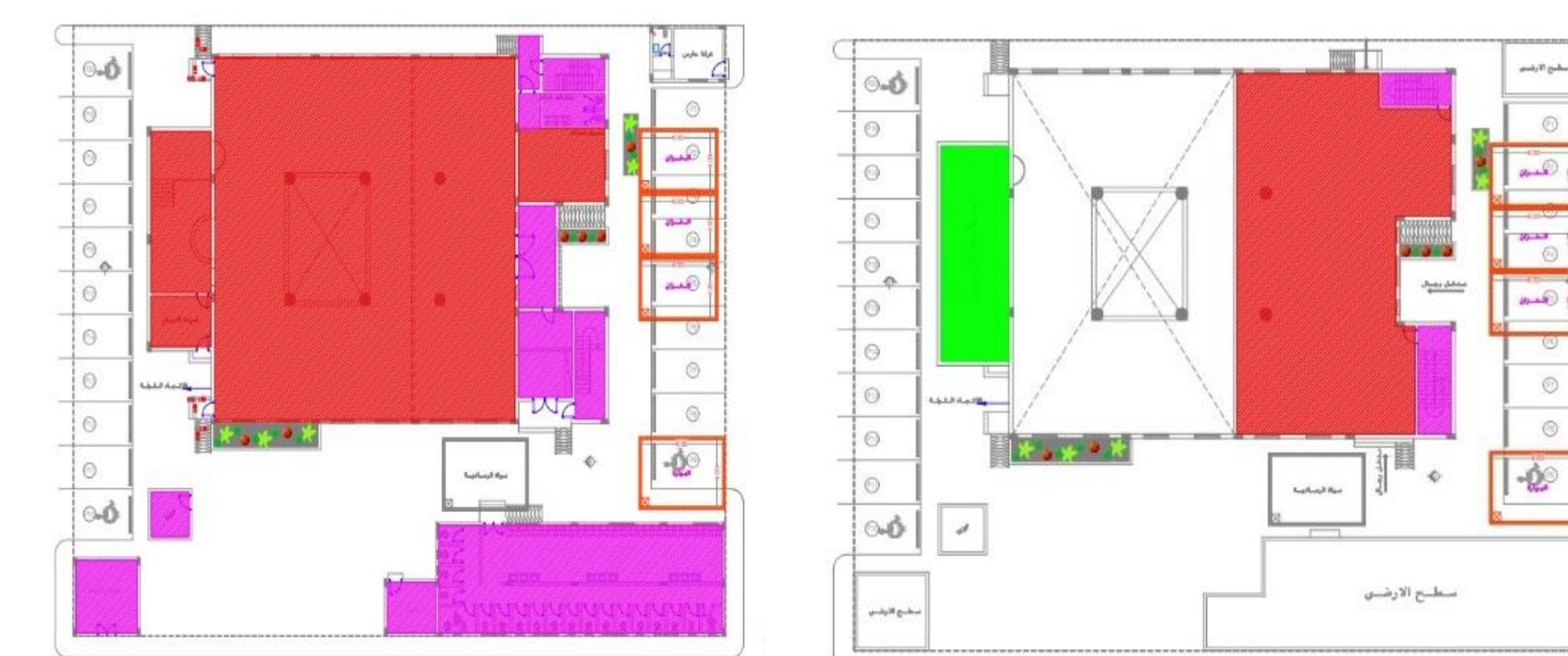
Figure.3 AC distribution in ground and first floor
