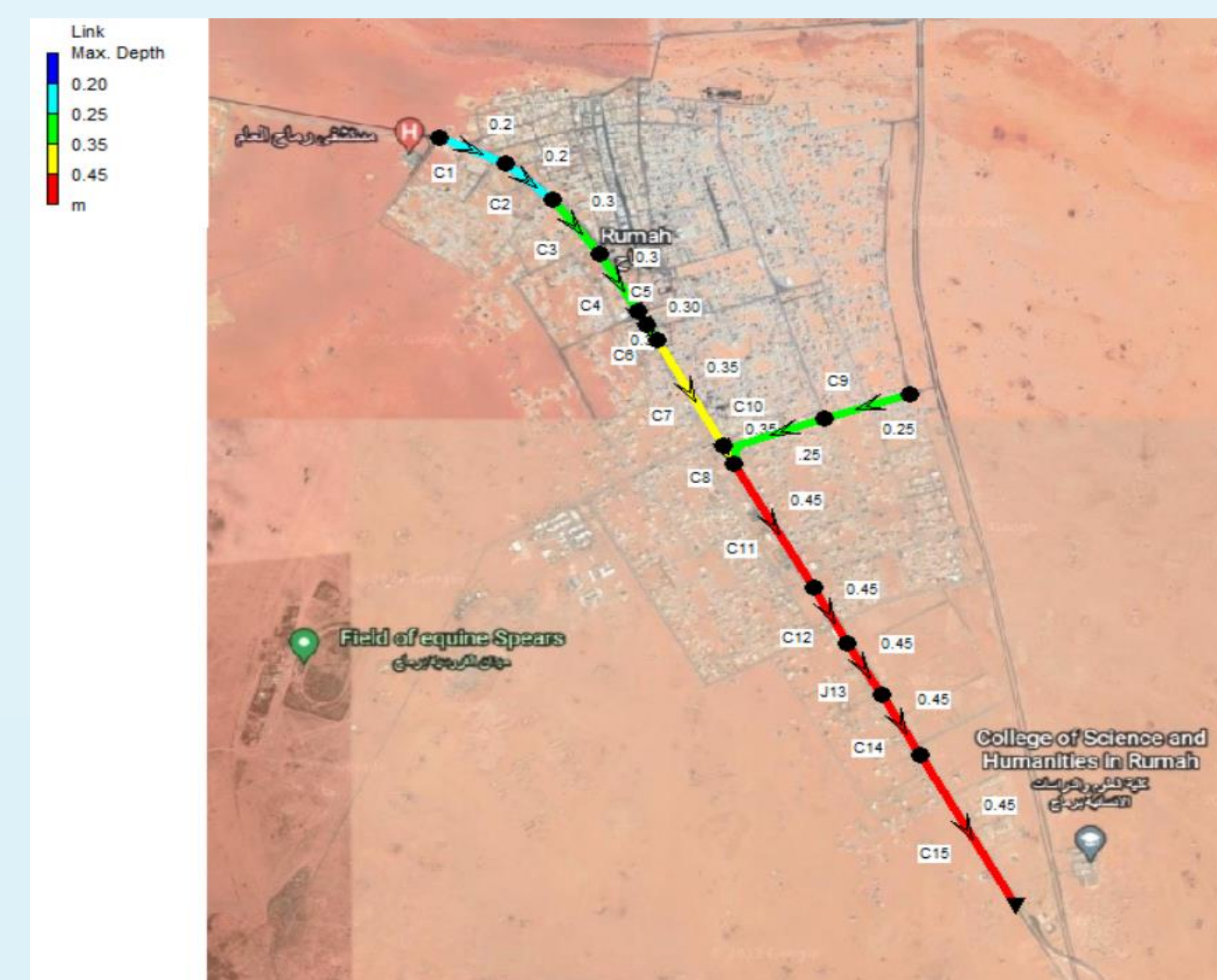
Figure 3.3 Diameters of conduits
