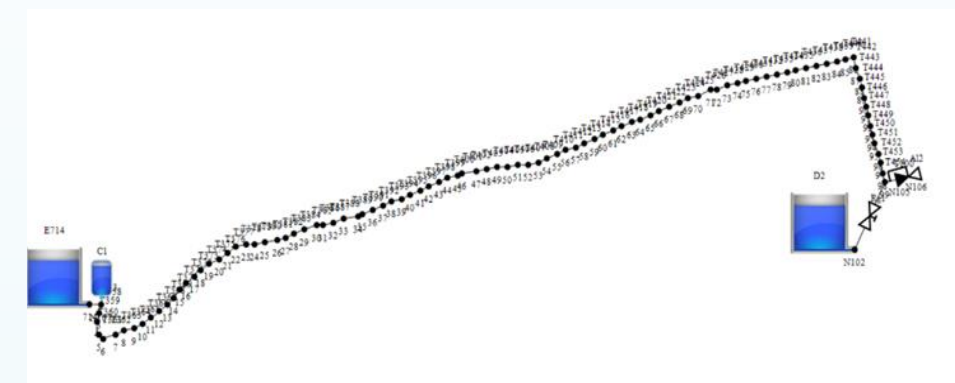
pipe transmission line from Allievi ( first 50 km )
