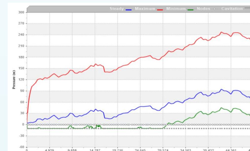
Max and Min Pressure Envelopes of Water Hammer using Allievi Due to valve closure ( Tc = 16 sec ) ( without Protection ) for first 50 km
