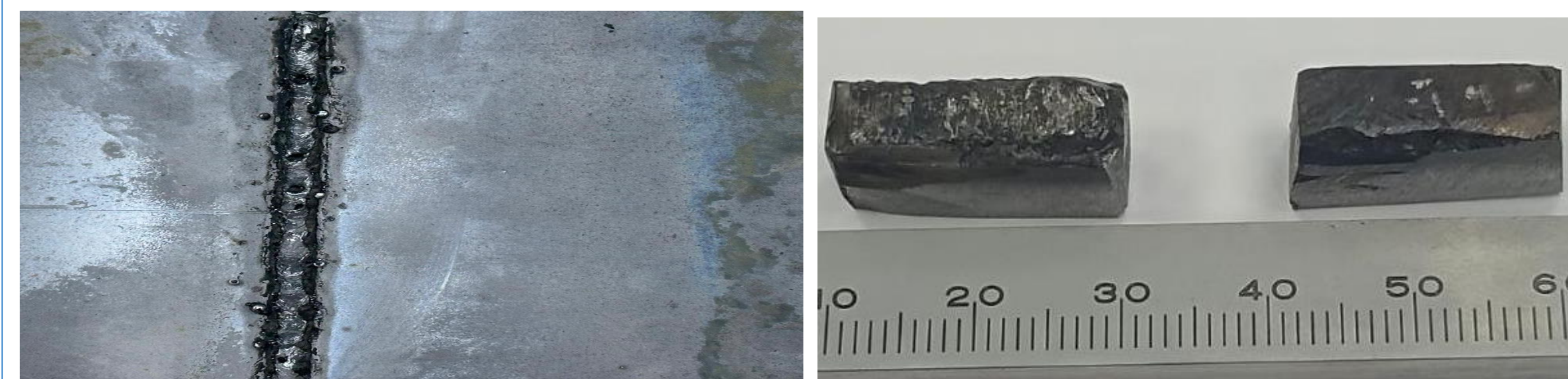
Figure 7: Welding in sea water condition, porosity
