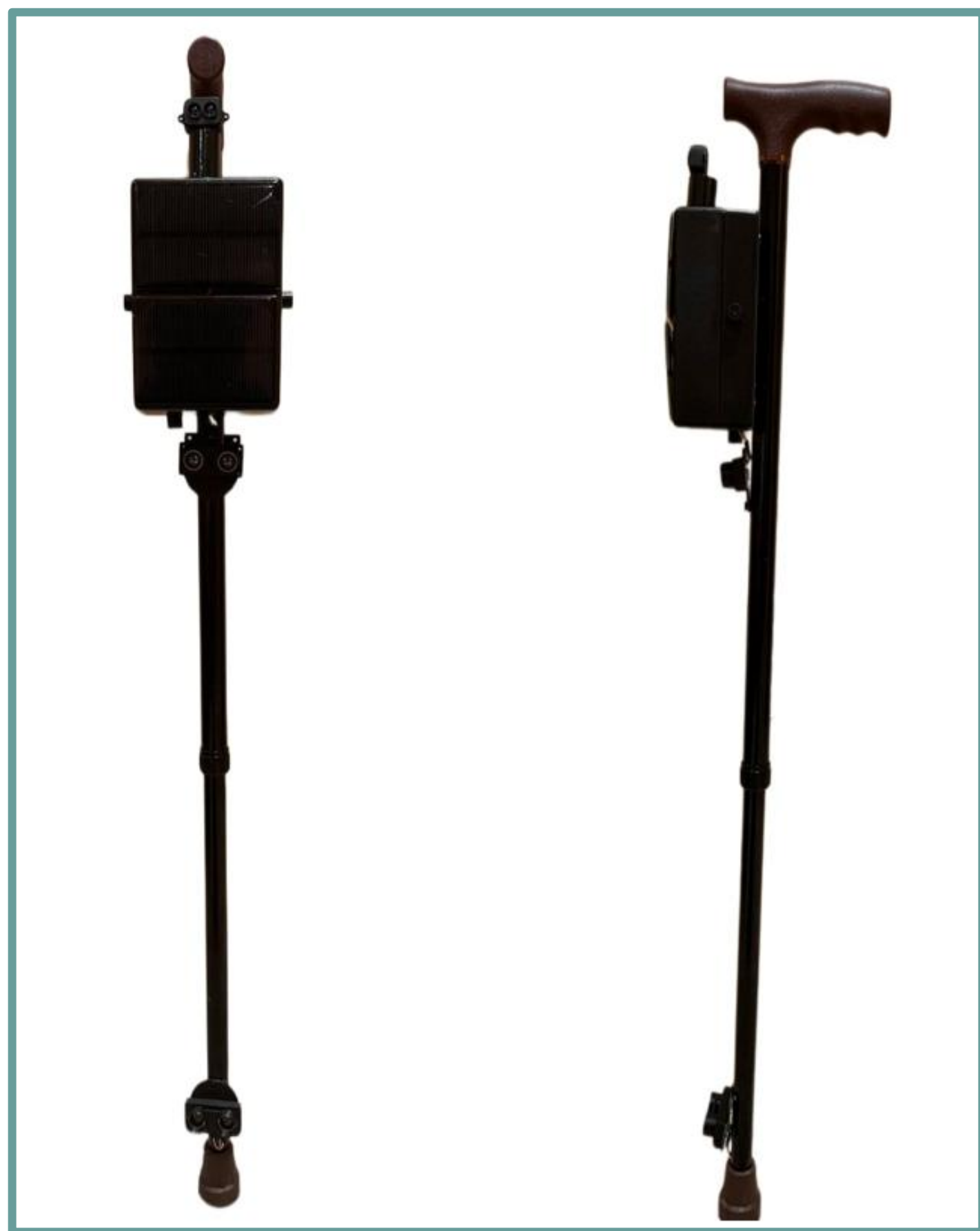
Front and side view of the design of the real solar smart stick.
