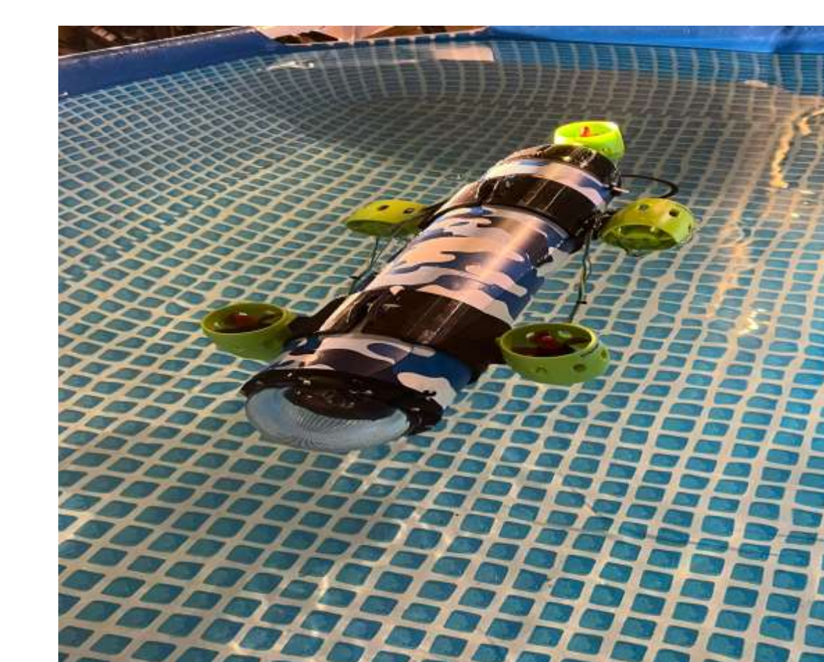
Figure 16: Testing ROV on Surface of The Water
