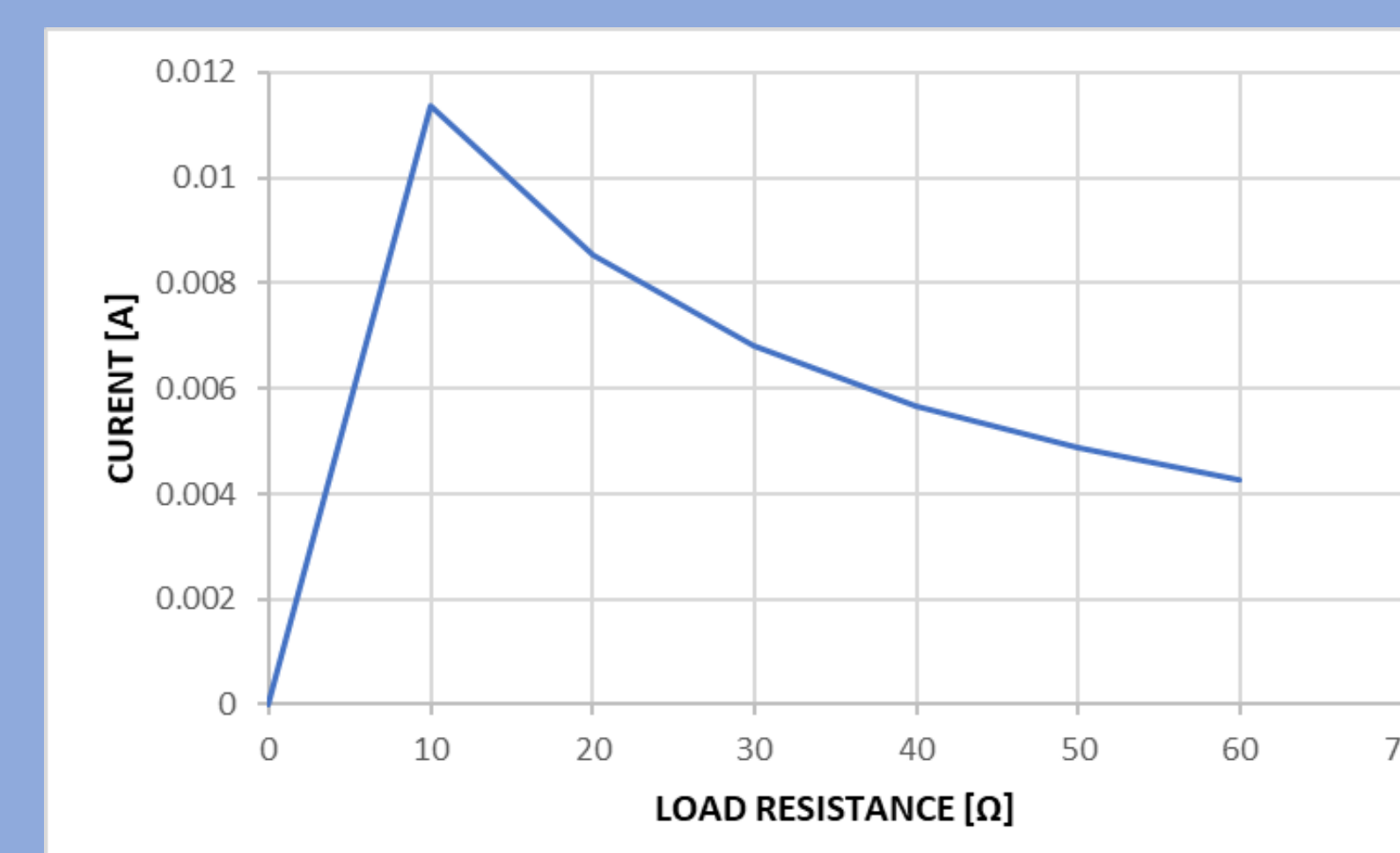
Figure 5 Current vs load resistance for multi-couple TEG
