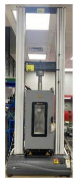
Figure 1. Tensile Testing Machine Type Instron, Model: 3367, maximum load 30 kN.
