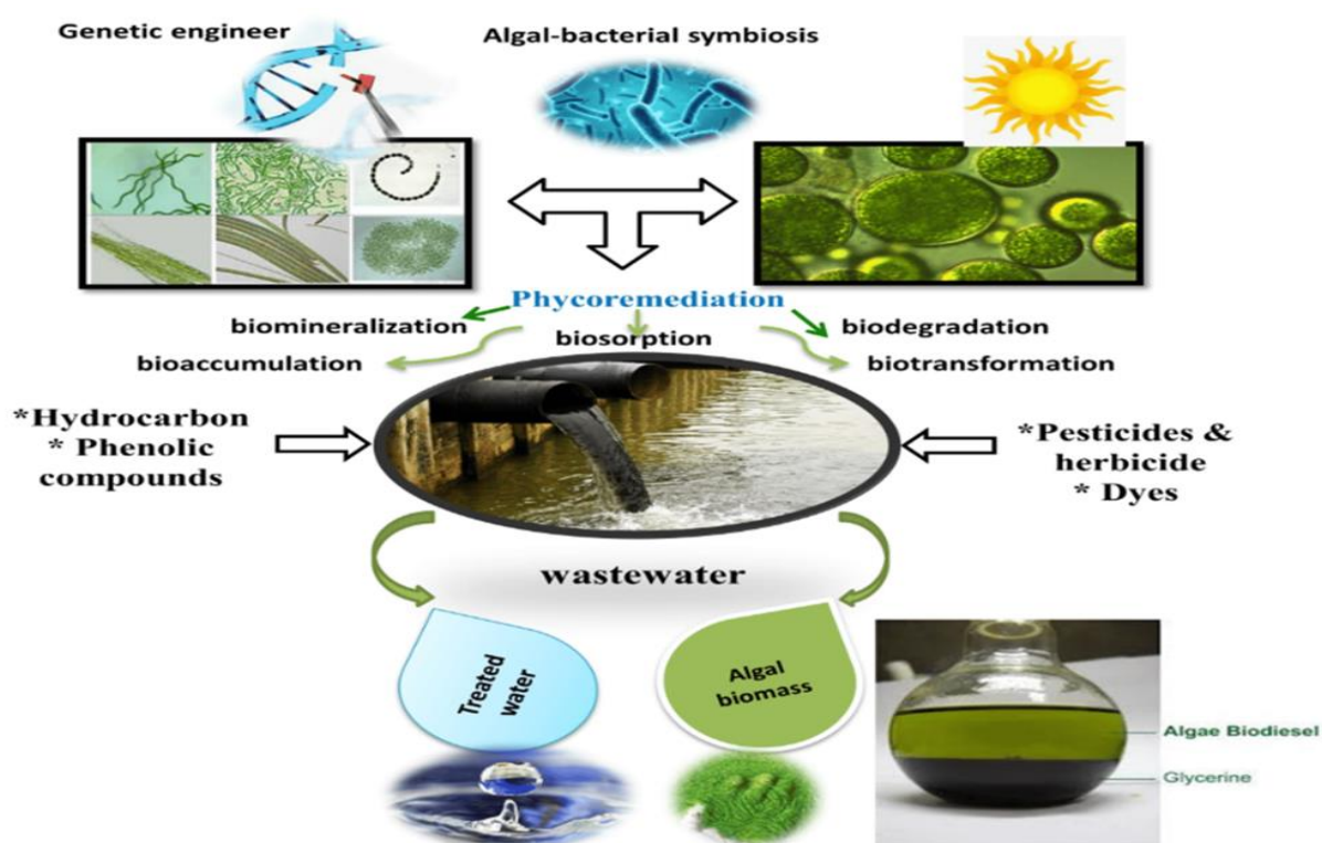
Fig.11. Phytoremediation of organic pollutants by microalgae, cyanobacteria, and biomass utilization (Touliabah et al. , 2022).
