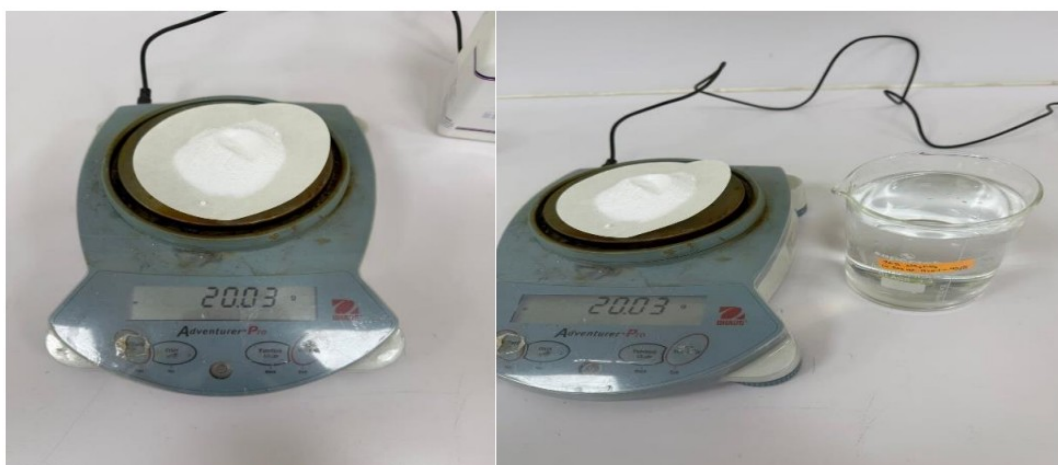
Figure (3.4): Measurement 20g of \text{Na}_2\text{CO}_3 in 500ml of \text{H}_2\text{O}
