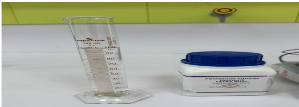
Figure (3.5): measurement 1g of \text{KNaC}_4\text{H}_4\text{O}_6 \cdot \text{H}_2\text{O} in 100ml \text{H}_2\text{O}
