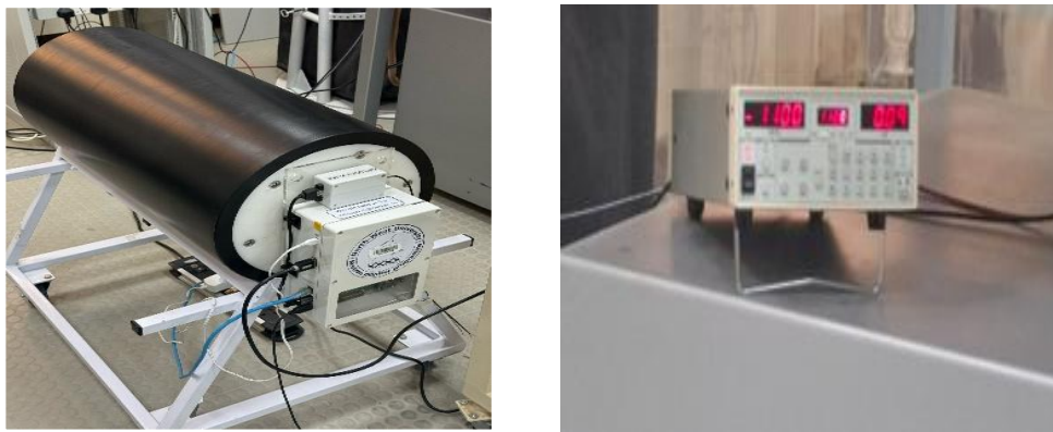
Figure 2.2: The mini neutron and muon monitor installed at the KACST station.
