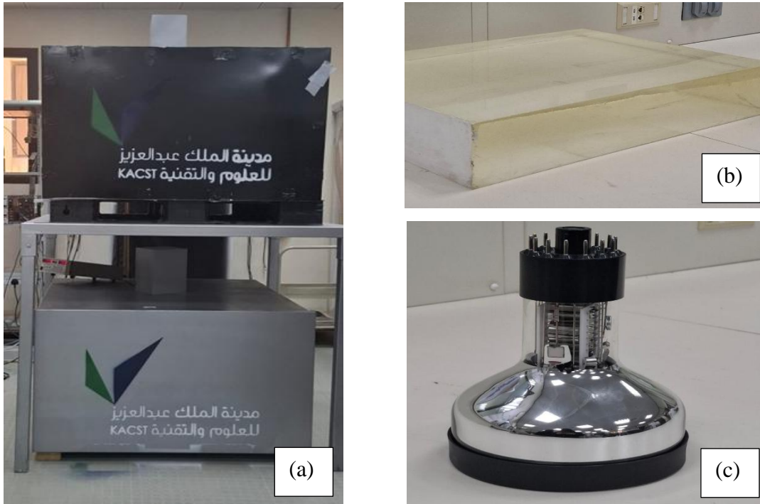
Figure 2.1: (a) The upper and lower detectors stacked on top of each other, (b) scintillating crystals used within the detectors, (c) the photomultiplier tubes.
