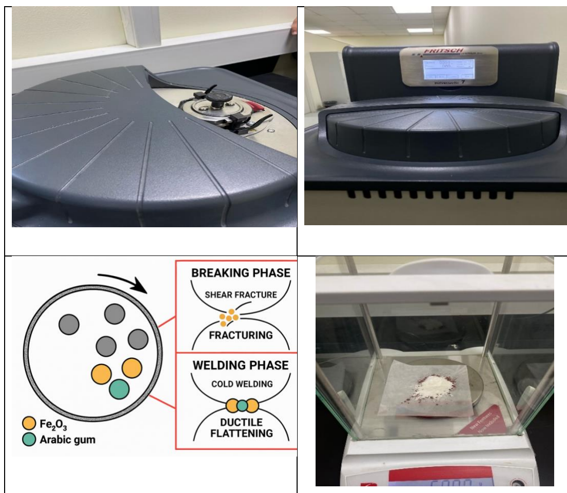
Figure.2.2: Schematic diagram for the preparation of nano alloys using ball milling
