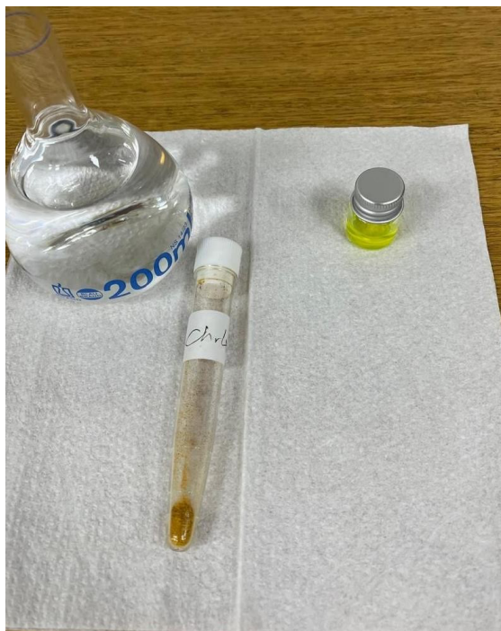
Figure 3.1 Image of 2mg of Chr2 dissolved in 4ml of acetone
