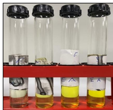
Fig 4.6 Chalcone in in Ethyl acetate for different concentrations
