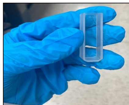
Fig 4.8 The quartz cuvette used for the absorption measurements
