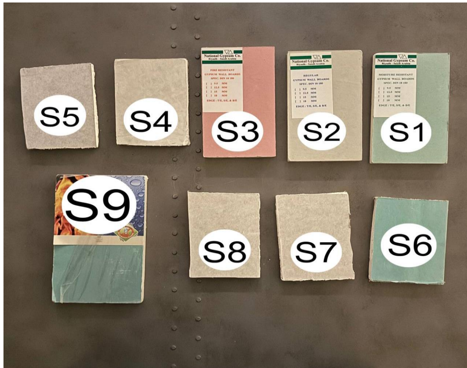
Figure 3.1: Gypsum board samples used in the experiment
