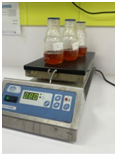
Figure 2.3: Image showing the heating of iron salt solution.
