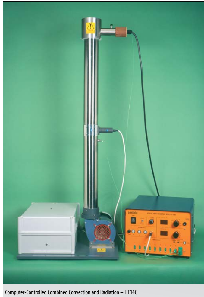
Computer-Controlled Combined Convection and Radiation – HT14C
