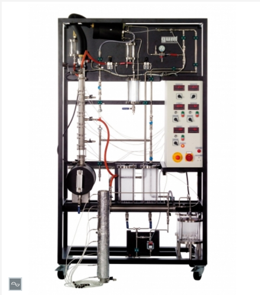
The illustration shows the CE 600 with built in sieve tray column. The packed column can be seen in the foreground.
