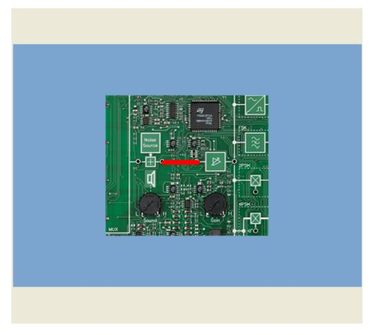
In the following experiment we will investigate detection of single-bit errors when a single parity bit is used. The bit error generator on the COM3LAB is used to generate the bit errors. Since the actual transmission is undisturbed (no noise), data formatting and type of modulation do not matter; in this example NRZ format and ASK are used.
