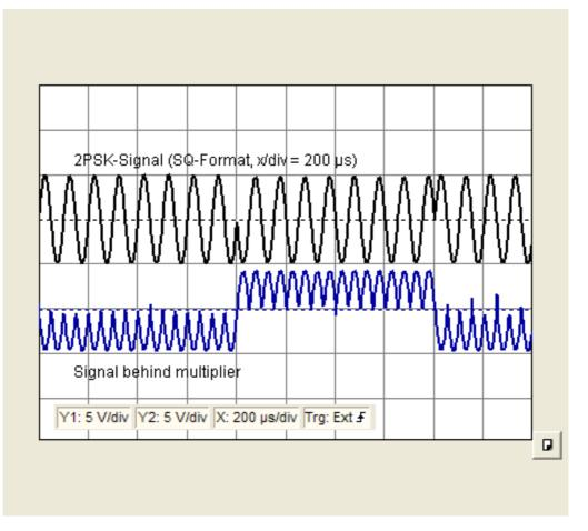
The first thing you notice is the effect of the multiplication by the frequency- and phase-identical carrier signal. The low-pass filter results in a signal with an e-shaped, rising (bit logical 1) or falling (bit logical 0) edge. The Schmitt trigger generates the actual data signal from that, which due to the effect of the low-pass and Schmitt trigger is shifted by around 120  $\mu$ s from the original signal.
