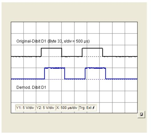
Since 4PSK demodulation consists essentially of two separate 2PSK synchronous demodulators, you get for the individual dibits identical ratios and signal courses as for 2PSK demodulation. The original and demodulated dibit are each shifted by around 120  $\mu$ s due to the effect of the low-pass filter and Schmitt trigger.
