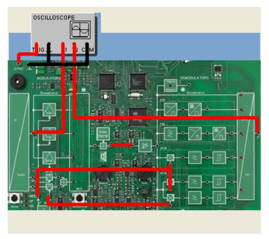
In the following experiment we will investigate the effect of the noise level on the bit error rate with Frequency Shift Keying (FSK) and Four-Phase Shift Keying (2PSK and 4PSK<sup>1</sup>) and compare the relationships with Amplitude Shift Keying. To exclude the effect of carrier recovery in 2PSK and 4PSK demodulation, the original carrier signal is used in these cases for demodulation.
