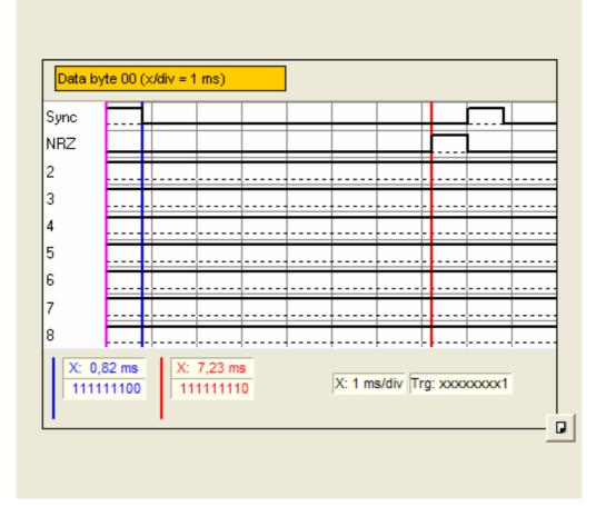
The curves show the expected structure of the signal consisting of the start bit<sup>1</sup>, data bits<sup>2</sup> (between the blue and red cursor) and the stop bit<sup>3</sup> (logical 1, to the right of the red cursor). After the start bit follows first the least significant bit (LSB), then the higher value data bits. For the total of ten bits (start bit, stop bit, eight data bits) a transmission time of 8 ms is required. This results in a bit rate of 10 • 1000 / 8 = 1250 bps.
