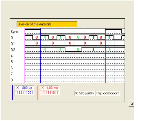
To the right of the blue cursor is the data signal D with first the digit 5 of the data byte 45 (LSB first), then the four bits of the digit 4. These end at the stop/start block at the same time as the sync signal (red cursor). You can see how the start bit, the eight data bits (between blue and red cursor) and the stop bit are "divided" over the two dibit signals. In this case 3.2 ms are required for transmitting the data bit. The bit rate is therefore
