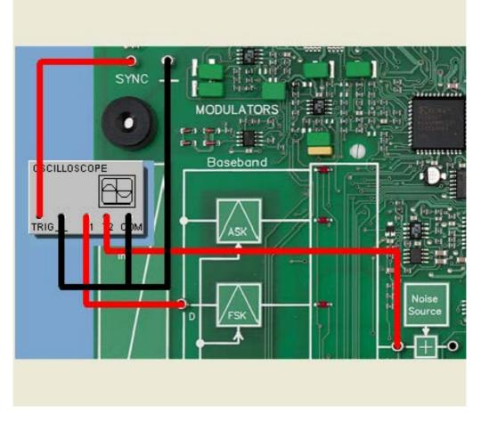
In the following experiment we will again study the modulated signal in two-phase shift keying, whereby the data signal will now consist of continuously varying data in NRZ and DIF format. The COM3LAB Spectrum Analyzer is again used to determine the spectrum.
