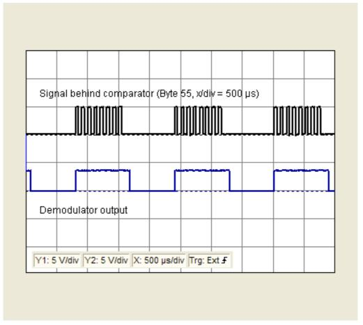
The ASK-modulated signal consists - as previous experiments have shown - consists of an amplitude of 0 for a bit at logical 0 and eight sinus oscillations for a bit of logical 1. Behind the comparator there is thus a sequence of eight pulses at TTL level for a bit with logical 1. The re-triggerable monoflop forms the original data bit from these individual pulses.
