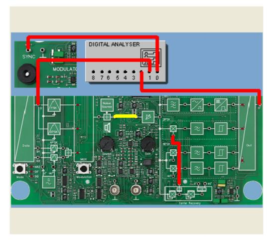
In the following experiment we will investigate the demodulation of a 2PSK modulated signal, whereby the reference carrier is recovered from the modulated signal on the receiver side. A data byte of 01 will be sent periodically and the course of the signal recorded on the send and receive side.
