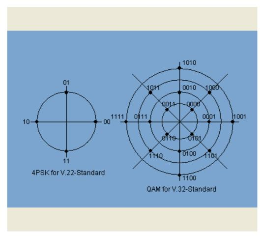
The various states in phase shift keying can also be shown very clearly in the form of vector diagrams, in which the angle of a vector represents the phase position of a state (for example of a dibit in 4PSK) and the length of the vector the amplitude (for example in quadrature amplitude modulation<sup>1</sup>). The adjacent graphic shows two examples.
