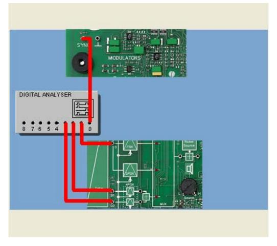
In the following experiment we will investigate the principle of dibit generation through serial-to-parallel conversion. A suitable data byte will be periodically generated and the resulting dibit signals  $D_1(t)$  and  $D_2(t)$  recorded with the help of the digital analyzer. From the courses we will then determine the transmission rate for four-phase shift keying.
