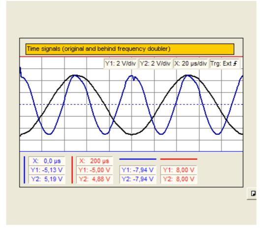
The first quadrupling results in a sinusoidal signal having frequency 2  $f_0 = 20$  kHz, the second quadrupling in a signal with a frequency of 4  $f_0 = 40$  kHz; the corresponding spectra thus consist only of a single line. The frequency divider reconstructs the signal into a (square-wave) signal having frequency  $f_0$ , which also has low-amplitude harmonics at odd multiples of the carrier frequency, in other words at 30 kHz, 50 kHz, 70 kHz etc.
