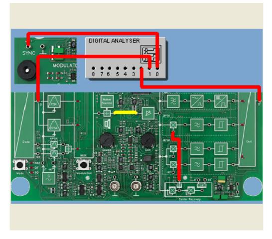
In the following experiment we will by way of comparison investigate the demodulation of a 2DPSK modulated signal, whereby the reference carrier is again recovered from the modulated signal on the receiver side. A data byte of 01 will be sent periodically and the course of the signal recorded on the send and receive side.
