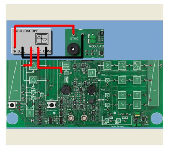
In the following experiment we will deepen our understanding of the 4PSK spectrum with square-wave modulation by investigating the composition of the spectrum made up of the two 2PSK spectra, in other words the spectra of the carrier signals modulated over the dibit signals  $D_1$  and  $D_2$  and shifted by 90° (inphase modulator and quadrature phase modulator). A square-wave signal (SQ format) will again be used as the modulating signal.
