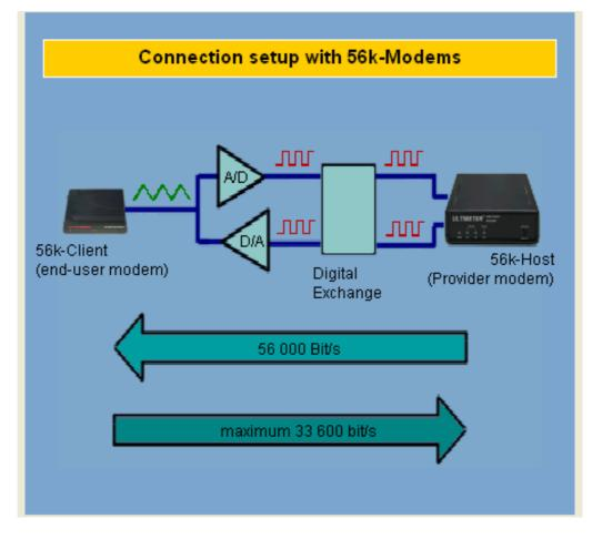
Modern 56k modems allow - even if only in the host-to-client direction - transmission rates to be achieved which are theoretically not possible for pure analog technology according to the Shannon Theorem<sup>1</sup> and the bandwidth of the telephone network, which is limited to around 3.1 kHz. This is accomplished by configuring one end of the transmission channel digital and in the analog part sending analog signals directly instead of a digitally modulated signal.
