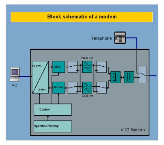
The modulator and demodulator form the core components of a modem. In addition, a modern modem has a variety of additional components which are responsible mainly for control of the modem and switching between the send and receive channel. The adjacent graphic shows a detailed block schematic of a modem.
