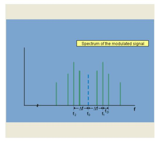
The frequency-shifted signal can be interpreted as the combination of two amplitude-shifted signals having frequencies
