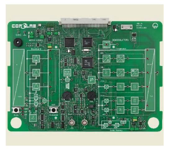
The COM3LAB-Board 700 74 Modem Technology contains all the components needed for an introduction to digital modulation. This includes especially modulators for amplitude, frequency and two- and four-phase shift keying as well as the corresponding demodulators. Data transfer can be performed over various channels which can be noise induced using an integrated noise generator.
