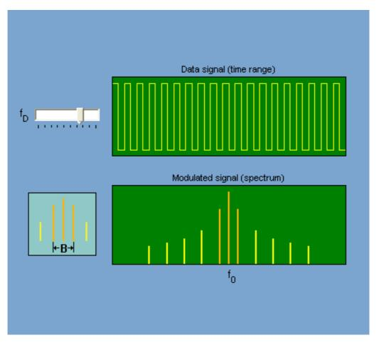
For unambiguous detecting of the signal state on the receiver side, it is sufficient if the spectrum is transmitted up to the first pair of side-bands, in other words in the range  $f_0 - f_D \dots f_0 + f_D$ . The theoretical minimum required bandwidth<sup>1</sup> is therefore
