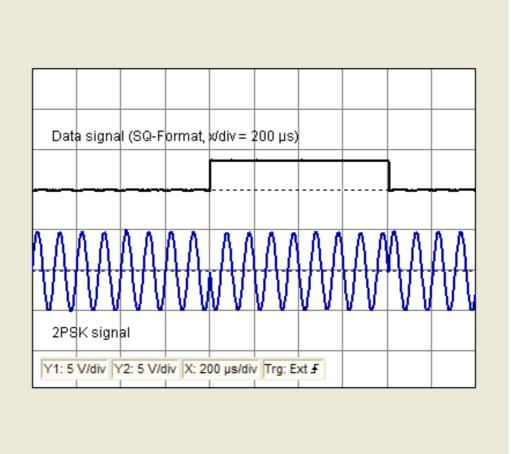
With the selected square-wave data signal alternating LOW and HIGH pulses are sent; each has a duration of 800  $\mu$ s (upper curve). The frequency of the carrier is constant at a value of 10 kHz. For a data bit of logical 0 the carrier has a phase shift of 0°, and for a data bit of logical 1 a phase position of 180°.
