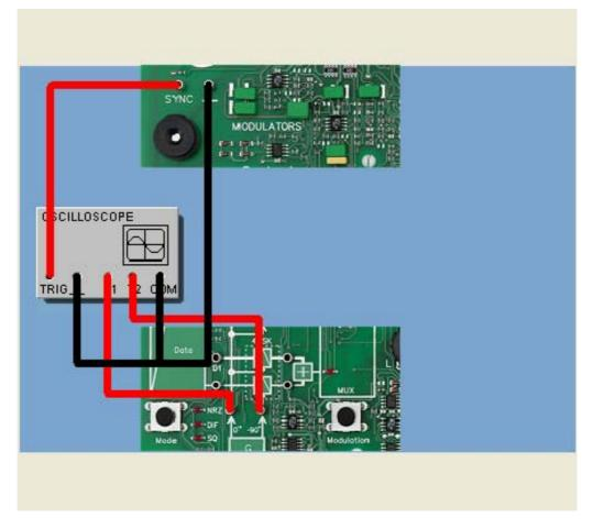
In the following experiment we will first study the courses of the two orthogonal carrier signals used in 4PSK. The courses will be captured by the oscilloscope and recorded both over time and in XY coordinates.
