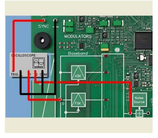
In the following experiment you will again study the amplitude spectrum of the modulated signal with amplitude shift keying, but now continuously different data in NRA or DIFF format will be sent as the data signal. The COM3LAB Spectrum Analyzer will again be used to determine the spectrum
