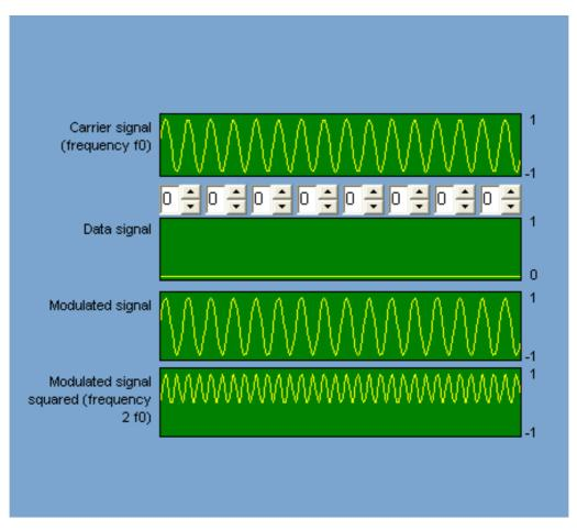
Since the carrier itself is not sent in 2PSK, it must be recovered in correct phase position for coherent demodulation at the receiving site. For this purpose the modulated signal can be squared; the result is a (DC component-containing) oscillation with double the carrier frequency, from which the carrier can be recovered by means of frequency dividing - though with a phase uncertainty of 180°.
