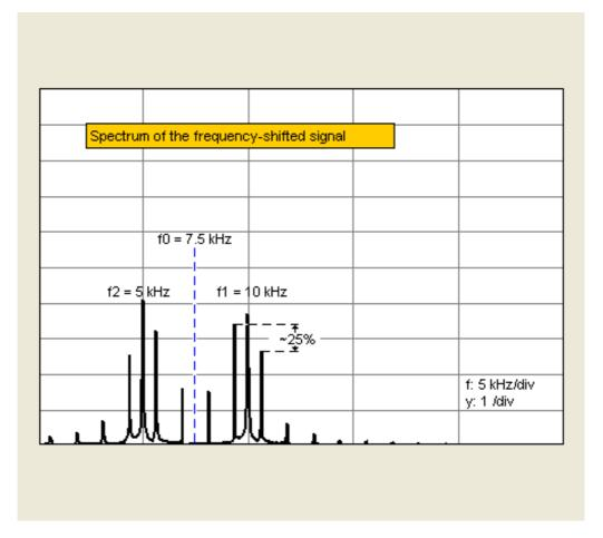
An amplitude spectrum symmetrical with respect to the center frequency of  $f_0 = 7.5$  kHz results, whereby the characteristic frequencies are at  $f_1 = 10$  kHz and  $f_2 = 5$  kHz. To the left and right of the characteristic frequencies are side-bands whose distances from the characteristic frequencies are each odd multiples of the data signal frequency  $f_D$ . Both "partial spectra' left and right of the center frequency are non-symmetrical with respect to the amplitudes of the side-bands.
