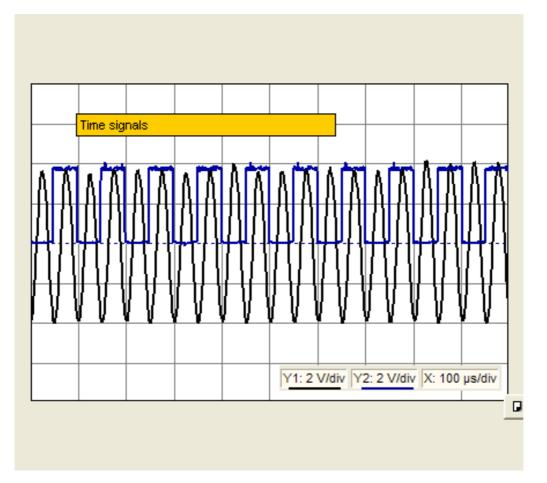
Multiplying the 2PSK signal by itself results in a purely sinusoidal signal with a frequency of 2  $f_0 = 20$  kHz, whose DC component is filtered out on the COM3LAB board. The frequency divider forms this signal into a square-wave signal with frequency  $f_0$ , which due to the square shape also contains harmonics at odd multiples of the carrier frequency, in other words at, 30 kHz, 50 kHz, 70 kHz etc.
