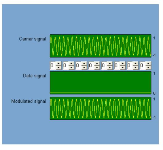
In two-phase shift keying  $(2PSK^1)$  a sinusoidal carrier signal with frequency  $f_0$  is toggled between two different phase positions depending on the data signal. Since disturbances generally affect only the amplitude of the signal and not its phase position, Phase Shift Keying is very noise-immune.
