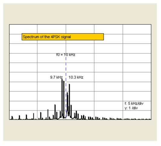
Four-phase shift keying works with double the bit rate as 2PSK, but the spectrum has about the same spread, in other words with the same bandwidth requirement 4PSK lets you send at double the bit rate. The carrier itself does not appear in the spectrum in 2PSK. Remark<sup>1</sup>
