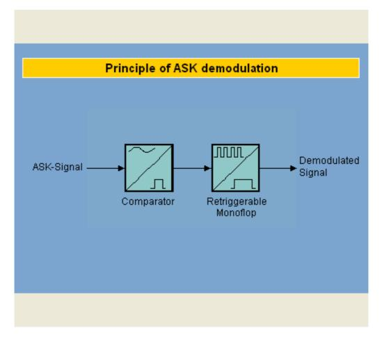
For demodulating<sup>1</sup> the ASK signal, envelope curve demodulation<sup>2</sup> is used. In the first step a comparator is used to hide the negative half-waves of the sinus oscillations and their amplitude is restricted to TTL level. In a second step a re-triggerable monoflop generates a single total pulse from the individual pulses belonging to a bit at logical 1; this total pulse then has the original length of the bit duration.
