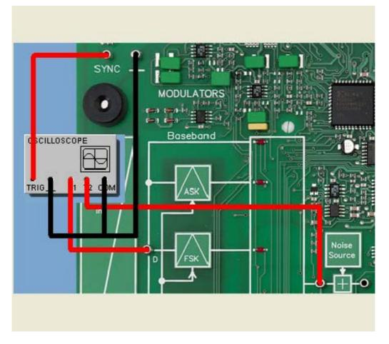
In the following experiment we will investigate the amplitude spectrum of the modulated signal in Four-phase Shift Keying. The data signal will again be a periodic square-wave signal<sup>1</sup> with a DC component and a frequency  $f_D = 600$  Hz.
