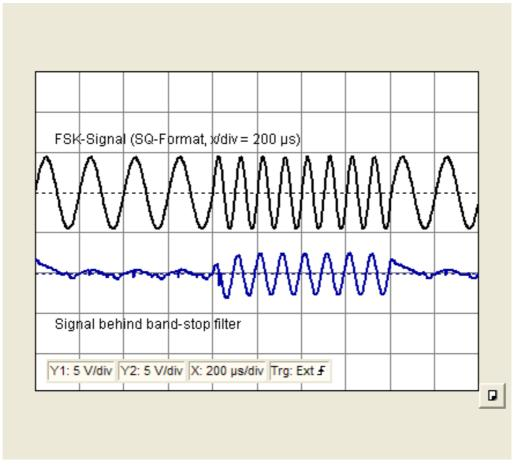
You can clearly see the effect of the band-stop filter: Whereas the upper frequency is only weakly damped, the amplitude of the lower frequency drops considerably. The band-stop filter also causes a phase shift in the signal however. Therefore there is a time delay of approx. 100 µs between the original data signal and the demodulated signal at the output of the FSK demodulator.
