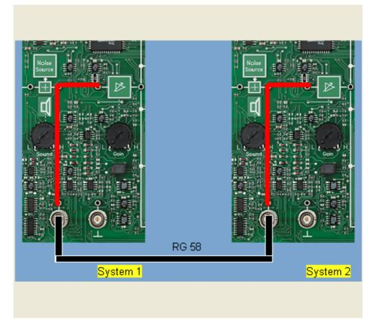
In the following experiment we will investigate half-duplex operation of two COM3LAB Master Units with the 700 74 Modem Technology experimenting board. Both boards will be connected here using a type RG 58 coaxial cable. Any desired texts are sent; transmission takes place without error checking and correction ('Parity' = none).
