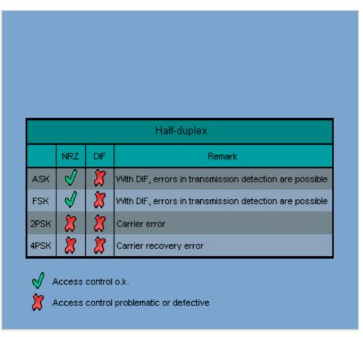
The channel access control implemented here in half-duplex detects the presence or absence of a carrier on the cable. Each station enables the channel after data transfer by turning off its carrier. The partner connected on the same cable detects the available carrier in the network and for its part activates its own sender. But as a result of unavoidable signal propagation times in the 'Signal Detect' stage, errors occur for individual modulation types (see table at right).
