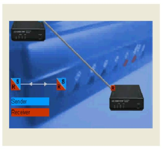
In half-duplex mode<sup>1</sup> the data are sent alternately in both directions over a common data line. At any given time this means that information only runs in one of the two directions, whereby the devices involved function alternately as a sender or receiver. Examples for half-duplex mode are short-wave (CB radio), walkie-talkies and intercom systems.
