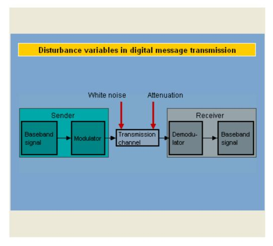
In addition to the energy and bandwidth requirement, freedom from errors in the transmitted information also plays an important role in digital message transmission. This can be expressed quantitatively by the bit error rate (**B**it **E**rror **R**ate BER<sup>1</sup>). Errorless message transmission is made more difficult on one hand by noise in the signal path, and on the other by signal attenuation by the transmission channel and the resulting deformation of the original bit pulses.
