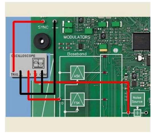
In the following experiment we will first study the modulated signal in two-phase shift keying. A periodic square-wave signal (SQ format) will be sent as the data signal and modulated on to the sinusoidal carrier signal. Both signals will be compared on the oscilloscope. Both the phase positions for logical 0 and logical 1 will be determined from the signals.
