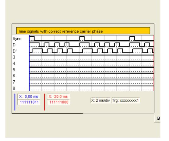
Here again, due to the phase uncertainty of the reference carrier of 180° there is a statistical phase error of just this 180° every second time the connection is opened. This results in the decoded data signal being exactly inverted on the receive side compared with the sent data signal. But with Differential Phase Coding this phase shift plays no role in data recovery, as will be shown in the following experiment.
