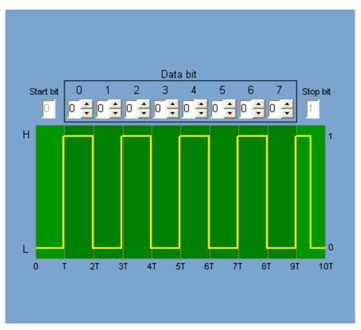
In Manchester format the transmission clock can be derived from the signal. At the start of each bit a signal edge (0-1 or 1-0 transition) is generated. For each bit having logical 1 an additional signal edge is also generated in the middle of the bit. The constant signal change gives the signal an AC voltage-like character in this format, giving it advantages with respect to what kinds of amplifiers can be used.
