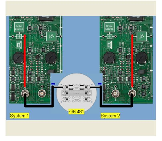
In the following experiment we will investigate simplex operation of two COM3LAB Master Units with the 700 74 Modem Technology experimenting board for sending over a transformer coupled twisted quad with amplitude shift keying in baseband. Any desired texts are sent; transmission takes place without error checking and correction ('Parity' - none).
