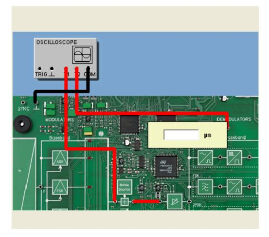
In the following experiment the access procedure to the common transmission channel in half-duplex mode will be investigated. The oscilloscope will be used to simultaneously measure and compare the modulated signal (her using ASK and NRZ format) and the output signal from the 'Signal Detect' stage.
