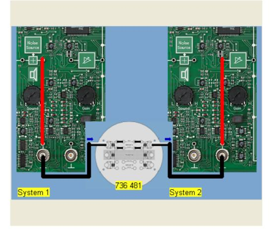
In the following experiment we will investigate simplex operation of two COM3LAB Master Units with the 700 74 Modem Technology experimenting board for sending over a transformer coupled twisted quad with four-phase shift keying in baseband. Any desired texts are sent; transmission takes place without error checking and correction.
