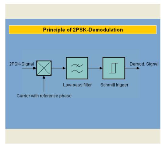
For synchronous demodulation of the 2PSK signal the carrier signal with the reference phase position is required. By multiplying with the 2PSK signal, the result is first a signal with double the carrier frequency whose center value over a bit width varies with the actual data bit. A downstream low-pass filter with pulse former (Schmitt trigger) finally regenerates the original data signal.
