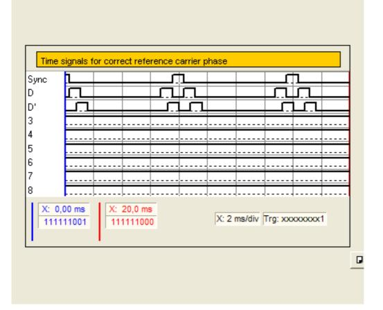
Due to the phase uncertainty of the reference carrier of 180° there is a statistical phase error of just this 180° every second time the connection is opened. This results in the decoded data signal being exactly inverted on the receive side compared with the sent data signal.
