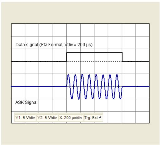
SQ format generates a square-wave signal with a pulse width of 800  $\mu$ s (upper curve), whereby the pulse width corresponds to the bit width. There are exactly eight oscillations of the carrier signal for each pulse (lower curve). The carrier signal thus has a frequency of  $f_0 = 10$  kHz.
