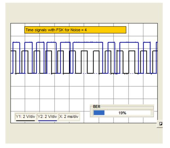
For FSK the theory is contradicted by worse results than for ASK, since the FSK demodulator in the COM3-LAB is based on prior ASK demodulation; FSK and ASK would be superior if more complex FSK demodulation were used. For 2PSK and 4PSK there are practically no bit errors at the observed noise level; PSK is the most noise-immune type of modulation. Even when the noise is raised to the maximum value the bit error rate remains practically zero.
