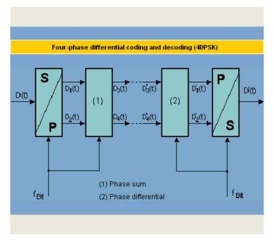
The phase uncertainty of the reference carrier of i • 90° with 4PSK can also be circumvented by using Differential Phase Coding, which in general functions in the same manner as 2DPSK. A digital phase adder (1) converts the dibit signals  $D_1(t)$  and  $D_2(t)$  into the differential encoded signals  $D_3(t)$  and  $D_4(t)$ . On the receive side a phase difference calculator (2) performs decoding of the dibit signals  $D'_3(t)$  and  $D'_4(t)$  into  $D'_1(t)$  and  $D'_2(t)$ .
