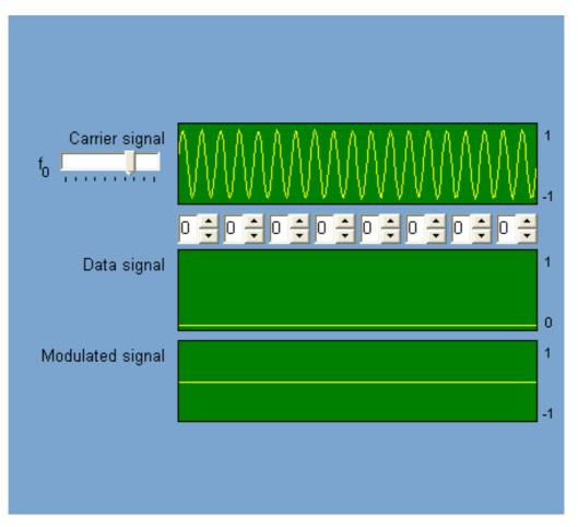
In Amplitude Shift Keying (Amplitude Shift Keying  $ASK^1$ ) a sinusoidal carrier signal having frequency  $f_0$  is turned on and off by the data signal (which is why this procedure is also known as ON/OFF keying). If the data signal has the value logical 1 (HIGH), the carrier signal is turned on, and a data signal of logical 0 (LOW) turns it off. ASK can therefore be implemented by means of a switch.
