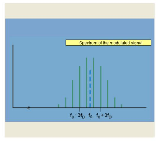
The spectrum of the 2PSK signal corresponds to amplitude modulation with suppressed carrier. The adjacent graphic shows the spectrum for modulation with a square-wave data signal having frequency  $f_D$ . As in the case of ASK, the minimum required transmission bandwidth is therefore
