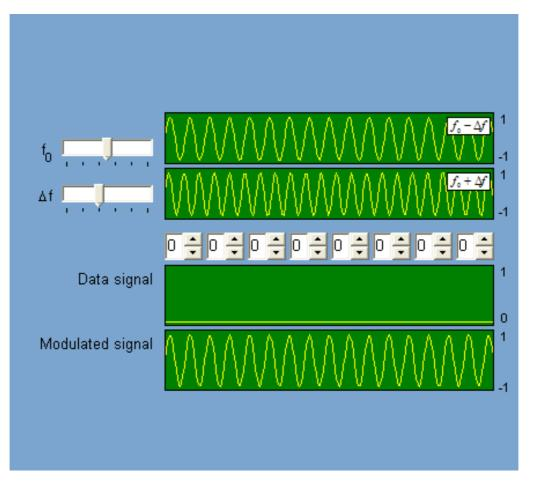
In Frequency Shift Keying (FSK<sup>1</sup>) depending on the data signal the shift is made between two frequencies  $f_0 - \Delta f$  (data bit is logical 0) and  $f_0 + \Delta f$  (data bit is logical 1). The frequency  $f_0$  is termed the center frequency<sup>2</sup>, the frequency  $\Delta f$  the frequency deviation<sup>3</sup>. Compared with ASK, FSK is significantly less noise-sensitive.
