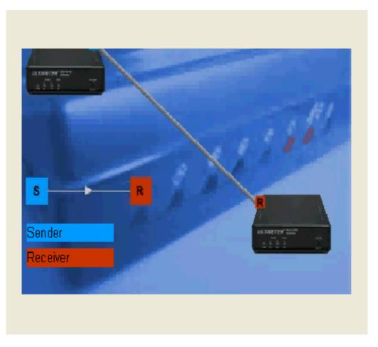
Depending on the transmission systems and the desired applications, there are various transmission types (direction modes) for the physical arrangement of data connections and the logical information flow over these connections. In simplex mode<sup>1</sup> data can be sent in only one direction from the data source (Sender S) to the data sink (Receiver R). Examples of simplex mode are radio and TV transmissions.
