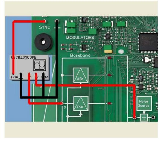
In the following experiment the amplitude spectrum of the modulated signal in Frequency Shift Keying will be studied, but now continuously varying data will be sent as the data signal in NRZ and DIFF format. The COM3LAB Spectrum Analyzer is again used to determine the spectrum.
