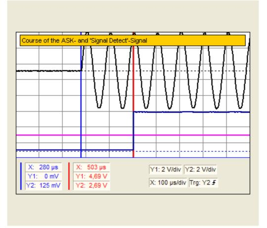
The output signal of the ,Signal Detect' stage is a square wave jump and appears after the ASK-modulated signal after a delay of about 220  $\mu$ s. This time delay is a critical phase in the half-duplex method of channel access control, since both partners detect the channel as available during this time.
