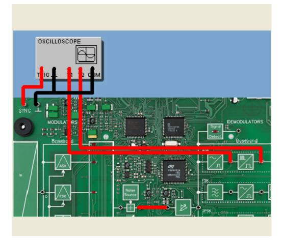
In the following experiment the demodulation of an ASK-modulated signal with NRZ formatting will be studied more closely. Periodically a data byte of 55 will be sent and the course of the signal behind the comparator and monoflop of the ASK demodulator recorded. **Note:** Be sure that the ,Gain' adjustment is at full left for this and all following experiments.
