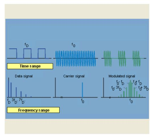
In the frequency range amplitude shift keying causes a shift of the data signal spectrum by the frequency  $f_0$  of the carrier signal. The graphic at the right shows this using the example of a periodic square-wave signal having frequency  $f_D$ . This signal has a line spectrum consisting of spectral lines with odd multiples of the base frequency  $f_D$ , in other words for the frequencies  $f_D$ , 3  $f_D$ , 5  $f_D$  ... The form of the spectrum itself is not changed by ASK.
