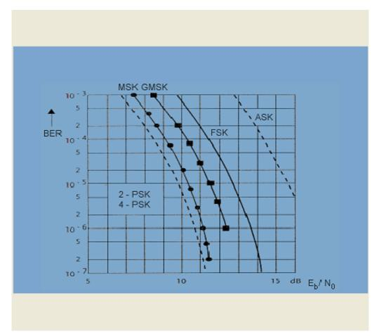
In addition to the formatting of the data in the baseband, the modulation procedure has an especially great effect on the bit error rate, as does the switching technique used in the modulator and demodulator. The adjacent graphic shows the bit error rate for the procedures under discussion as a function of the quotient  $E_b/N_0$  as a measure of the signal-to-noise ratio ( $E_b$ : Energy per bit,  $N_0$ : Noise power density at the receiver).
