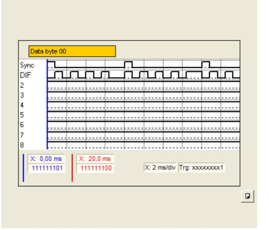
With a data byte of 00 the signal level changes with each data bit; with a data byte of FF it remains constant. With a data byte of 55 the level changes with each second data bit. Since the start bit has the value logical 0, the signal level changes at the beginning of each bit sequence. This results in every second bit sequence being sent inverted (you can see this especially clearly with FF).
