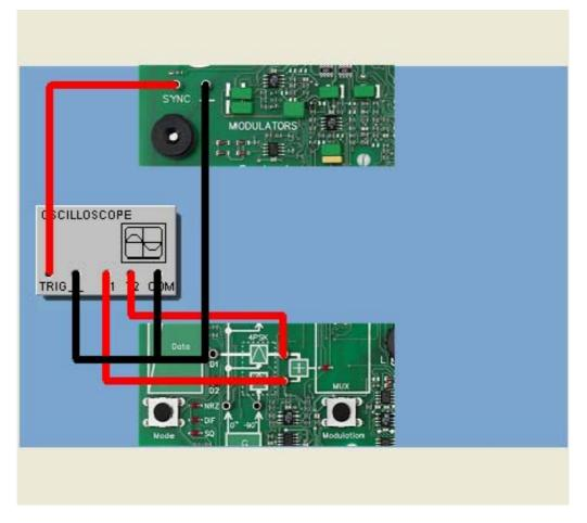
In the following experiment we will analyze the composition of the 4PSK signal made up of the two 2PSK signals. A data byte of 03 will be sent periodically. The courses of the two 2PSK signals will be captured with the oscilloscope.
