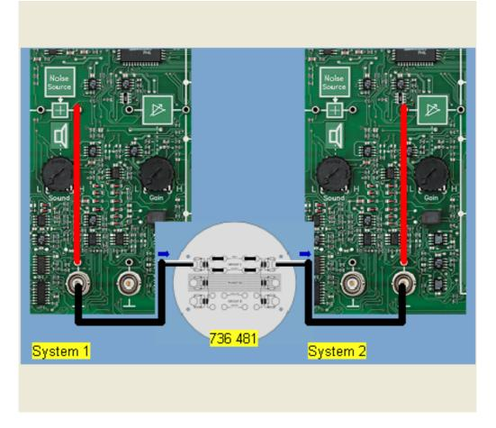
In the following experiment we will investigate simplex operation of two COM3LAB Master Units with the 700 74 Modem Technology experimenting board for sending over a transformer coupled twisted quad with two-phase shift keying in baseband. Any desired texts are sent; transmission takes place without error checking and correction ('Parity' - none).
