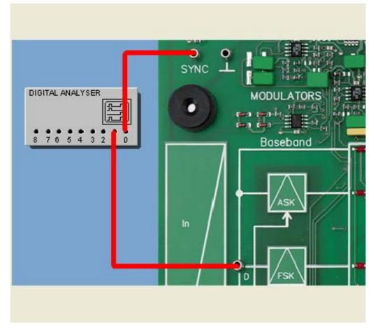
In the following experiment you will study the differential data format more closely. Periodically differing data bytes will be transmitted and the course of the encoded data signal will be recorded with the digital analyzer. The obtained signals will be compared with those of the NRZ encoding.
