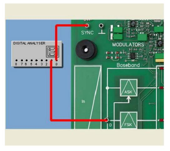
In the following experiment you will study the NRZ data format in greater detail. Periodically different data bytes will be transmitted and the curve of the encoded data signal recorded with the digital analyzer. From the recorded curves the bit rate<sup>1</sup> of the data signal will then be determined.
