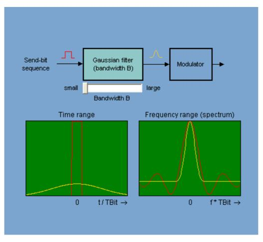
In Gaussian Minimum Shift Keying (GMSK<sup>1</sup>) further bandwidth limiting is accomplished by freeing the bit pulses from their steep pulse edges before modulation by means of a Gaussian low-pass filter (shape filter). Pulses filtered in this way then have the shape of a Gaussian bell curve, which can result in overlaying of successive pulses. On the receive side this means that greater effort is required for decoding the data signal when demodulating.
