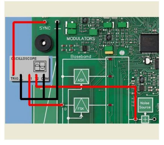
In the following experiment you will first study the modulated signal in amplitude shift keying. Periodically a constant data byte will be sent as a data signal and modulated on to the sinusoidal carrier signal. Both signals will be compared using the oscilloscope.
