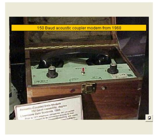
With the first modem types, the so-called acoustic couplers, the telephone receiver had to be placed in a special device in order to send the signal. In the meantime modems in a wide range of designs are available. Among the most important are external and internal models for use on a PC, which are connected to the serial port or plugged into a free ISA, PCI or PCMCIA slot in the computer.
