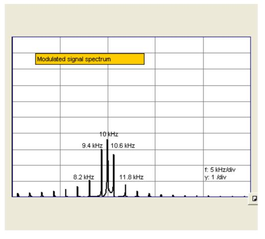
The spectrum of the data signal is shifted by the carrier frequency  $f_0$ ; the individual spectral lines appear mirrored left and right of the carrier. At  $f_0 = 10$  kHz the original data signal DC component thus appears, whereas the side-bands occur at the frequencies
