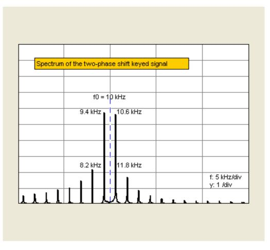
The result is an amplitude spectrum which is symmetrical with respect to the carrier frequency of  $f_0 = 10$  kHz, whereby the carrier itself no longer appears in the spectrum. To the left and right of the carrier frequency are side-bands whose separations are each an odd multiple of the data signal frequency  $f_D$  and whose amplitude decreases with increasing separation.
