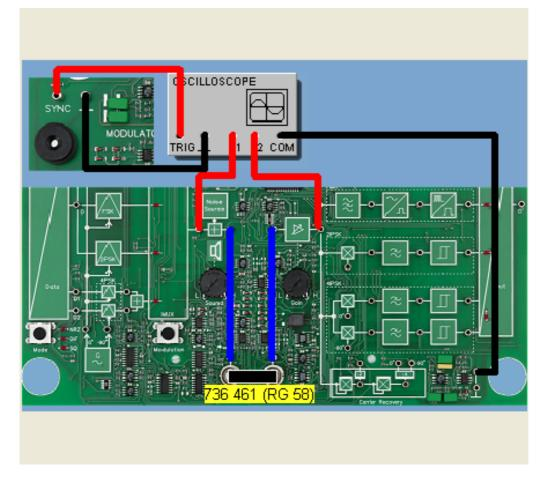
In the following experiment we will now investigate the influence of the transmission cable in Amplitude Shift Keying (ASK) and Frequency Shift Keying (FSK). A square-wave data signal will again be sent (SQ format) and the course of the signal recorded on the send and receive end. Two different coaxial cables as well as a twisted quad with differential transformer will be used.
