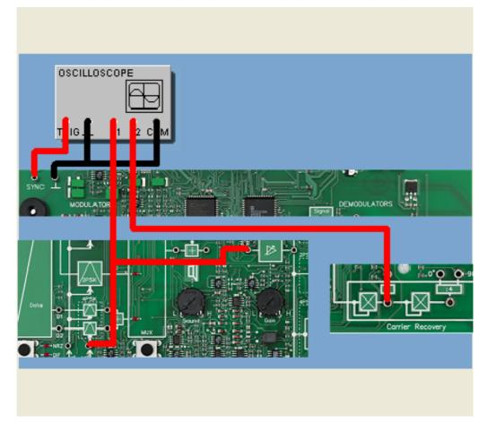
In the following experiment we will investigate carrier recovery with 4PSK whereby the modulated signal is squared twice. The analysis will be carried out in both the time and frequency range. Of particular interest are the signal spectra in front of and behind the frequency divider. To make the connections especially clear, the original carrier in 90°-position will be used as the "data signal".
