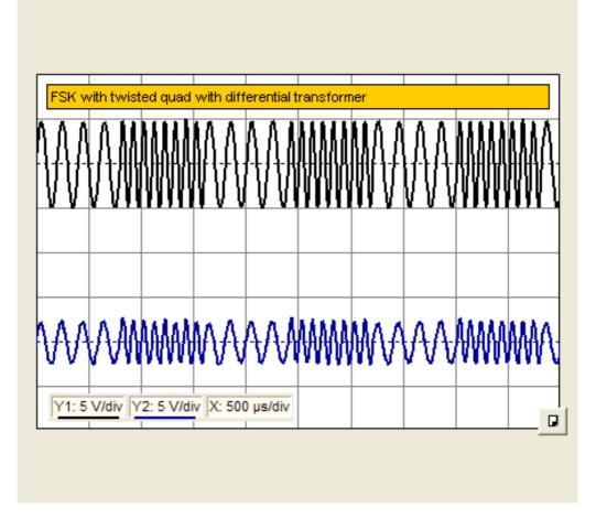
With ASK and FSK the baseband signal is shifted by the modulation to a frequency range around the carrier frequency  $f_0$ . In this frequency range all three studied cable types show only slight attenuation, so that except for the lower amplitude (which can be compensated by the receive-side amplifier) the receive signal is identical with the send signal.
