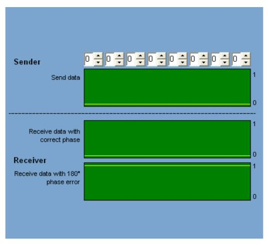
In carrier recovery with 2PSK there is a phase uncertainty of 180°, which can result in a mixup of the demodulated data bits (see illustration at right). This can be prevented by encoding a bit value not with the absolute value of the phase, but rather the phase differential from the previous value. This is referred to as Differential Phase Coding (DPSK<sup>1</sup>). Now a phase shift between sender and receiver carrier no longer plays a role.
