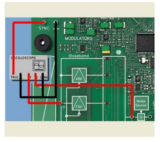
In the following experiment we will first study the modulated signal in frequency shift keying. Periodically a constant data byte will be sent as the data signal and modulated on to the sinusoidal carrier signal. The center frequency and frequency deviation can then be determined from the signals.
