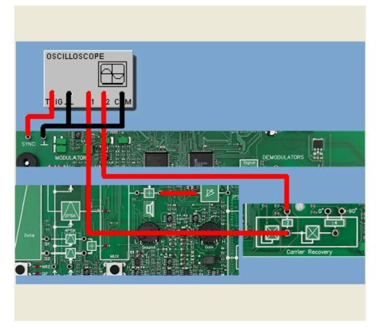
In the following experiment we will study carrier recovery with two-phase shift keying by squaring the modulated signal. The analysis will be made both in the time and frequency range. The data signal will again be a periodic square-wave signal with a DC component and a frequency of
