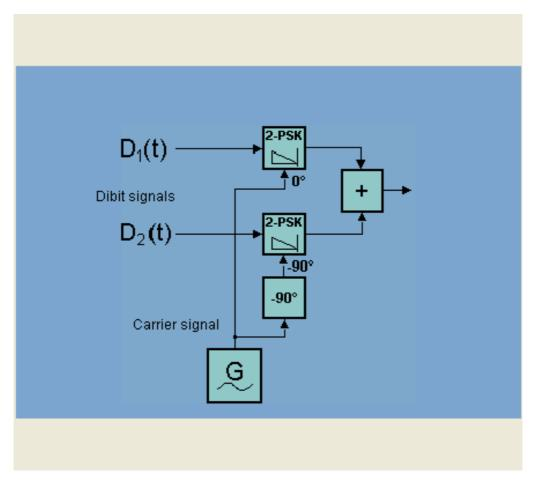
Four-phase Shift Keying is implemented with double, parallel Two-phase Shift Keying of the Dibit signals  $D_1(t)$  and  $D_2(t)$  with orthogonal carrier signals (phase position 0° and -90°) and summing of both signals. The 4PSK signal obtained in this way then has, depending on the bit combination present, phase positions of 45°, 135°, 225° and 315°.
