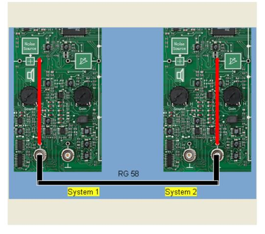
In the following experiment we will investigate simplex mode with two COM3LAB Master Units with the 700 74 Modem Technology experiment board. Both boards are connected here by way of example via a coaxial cable of type RG 58. Any desired texts are sent; transmission takes place without error checking and correction ('Parity' - none).
