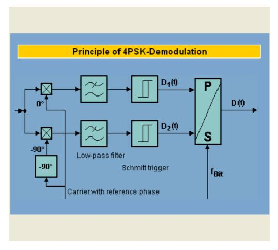
For synchronous demodulation of the 4PSK signal, two parallel 2PSK synchronous demodulators are used which work with  $-90^{\circ}$  shifted carrier signals. The resulting dibit signals  $D_1(t)$  and  $D_2(t)$  are restored to the total data signal D(t) in a parallel/serial converter.
