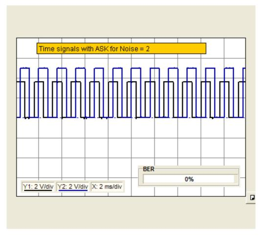
In this example with a noise level of 2 all the sent bits could be decoded without error on the receive side. The first bit errors begin to occur at a noise level of 4. The higher the noise level is, the more bit errors occur. You may get slightly different results do to manufacturing tolerances of the noise generator.
