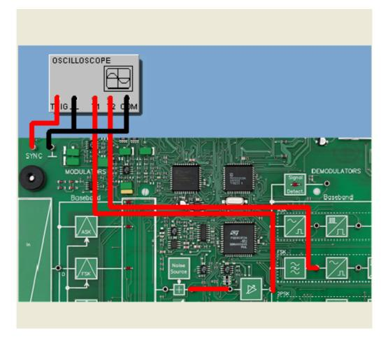
In the following experiment we will study the demodulation of an FSK-modulated signal in NRZ formatting more closely. A periodic square-wave signal (SQ format) will be sent and the signal trace recorded in the various stages of the FSK demodulator. The original data signal and demodulated data signal will then be compared.
