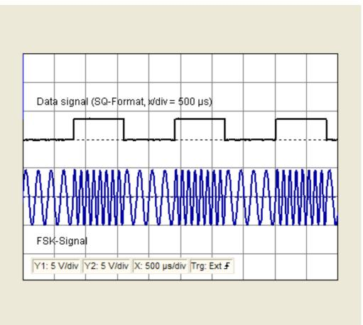
In SQ data format (symmetrical square-wave signal) alternating LOW and HIGH pulses are sent; each has a duration of 800  $\mu$ s (upper curve). At logical 0 there are four oscillations during this time, or eight at logical 1. This corresponds to frequencies of 5 kHz and 10 kHz. The center frequency is therefore 7.5 kHz and the frequency deviation 2.5 kHz.
