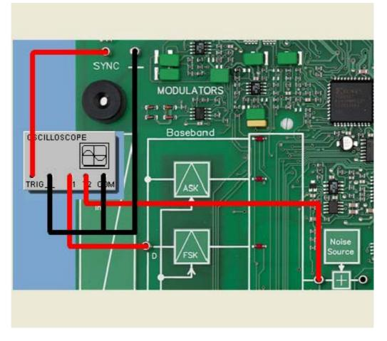
In the following experiment we will study the amplitude spectrum of the modulated signal in two-phase shift keying. As the data signal we will again use a periodic square-wave signal having a DC component (SQ format) and frequency  $f_D = 600$  Hz.
