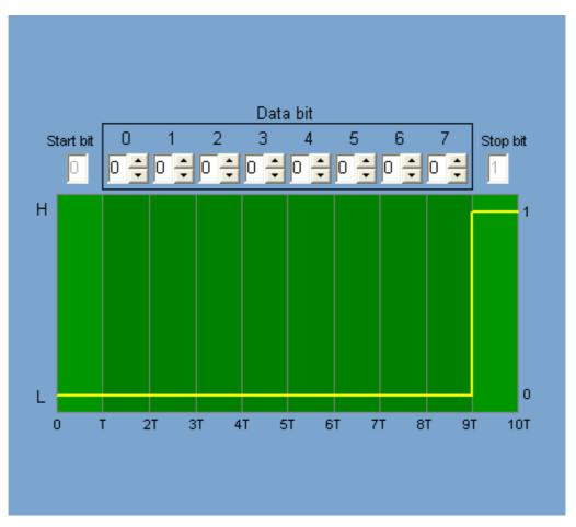
A general distinction can be made between synchronous<sup>1</sup> and asynchronous<sup>2</sup> transmission; only the latter will be considered in context of this course.
