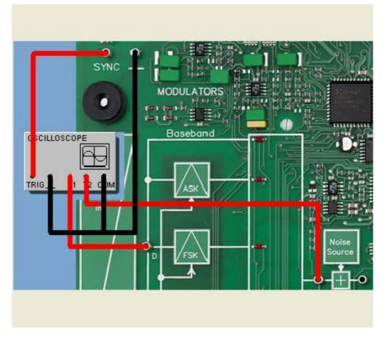
In the following experiment you will study the amplitude spectrum of the modulated signal in amplitude shift keying. A periodic square-wave signal having a DC component and generated by the SQ format will be used as the data signal. The COM3LAB Spectrum Analyzer will be used to obtain the spectrum; open the analyzer by clicking on the button  $\prod_{i=1}^{n}$ .
