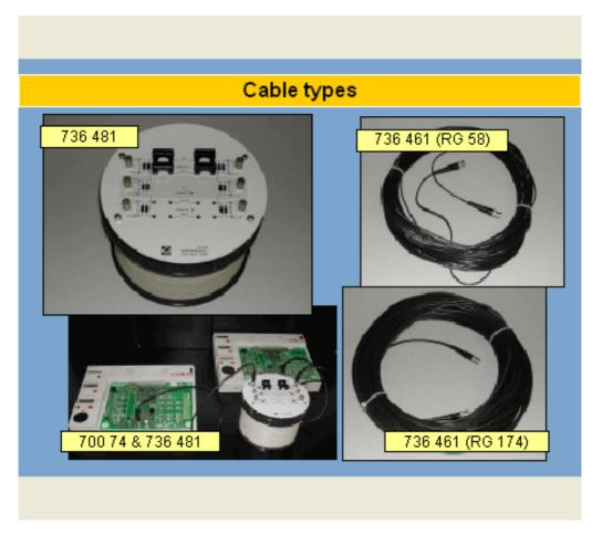
The communication channel - for land-line transmission this means the type of connection cable - has a significant influence on the quality of the data transfer. An improvement in transmission can for example be realized by refreshing the signal after a certain length of cable. In the following we will investigate various types of cables.
