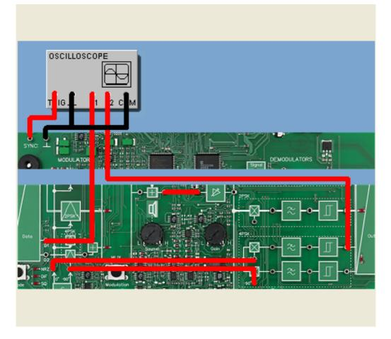
In the following experiment we will see that the 4PSK demodulator consists essentially of two separate 2PSk demodulators which each work with 90° shifted carriers. We will also investigate the demodulation of a 4PSK modulated signal in NRZ format, whereby periodically a data byte of 33 is sent. The original data signal and demodulates data signal will then be compared.
