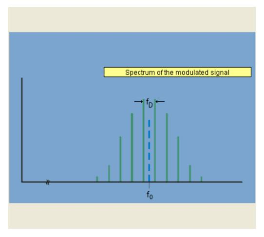
If four-phase shift keying is operated at the same bit rate as two-phase shift keying, a signal step has twice the duration. This reduces the spectrum as compared with 2PSK to half the width, as shown in the adjacent graphic for a square-wave data signal having frequency  $f_D$ . The minimum required transmission bandwidth is thus only
