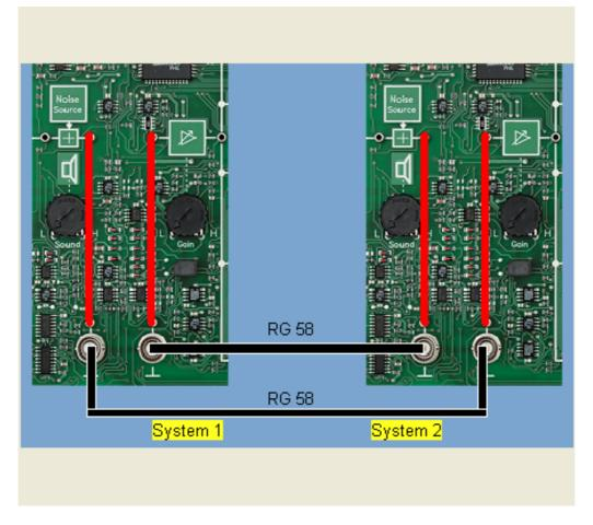
In the following experiment we will investigate full-duplex operation of two COM3LAB Master Units with the 700 74 Modem Technology experimenting board. Both boards will be connected here using a type RG 58 coaxial cable. Any desired texts are sent; transmission takes place without error checking and correction ('Parity' = none).
