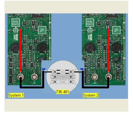
In the following experiment we will investigate simplex operation of two COM3LAB Master Units with the 700 74 Modem Technology experimenting board for sending over a transformer coupled twisted quad with frequency shift keying in baseband. Any desired texts are sent; transmission takes place without error checking and correction ('Parity' - none).
