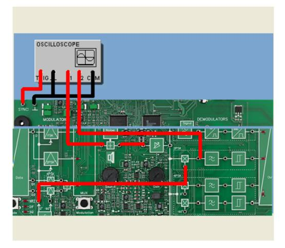
In the following experiment we will investigate in greater detail the demodulation of a 2PSK modulated signal with NRZ formatting. A periodic square-wave signal (SQ format) will be sent and the course of the signal recorded in the various stages of the PSK demodulator. The original data signal and demodulated data signal will then be compared.
