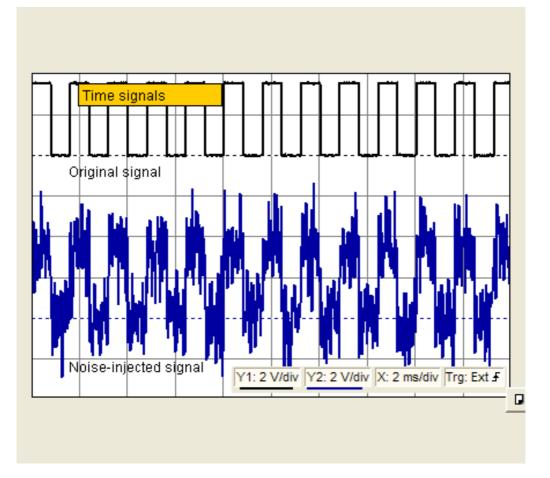
The noise generator approximates white noise, which is noise with a constant spectral power density over the entire frequency range. In the spectrum of the noise-injected signal this noise thus becomes apparent over the entire frequency range. Since statistically in the case of a square-wave modulation signal approximately every second bit is correctly recognized, the BER counter shows a maximum error rate of 50 %.
