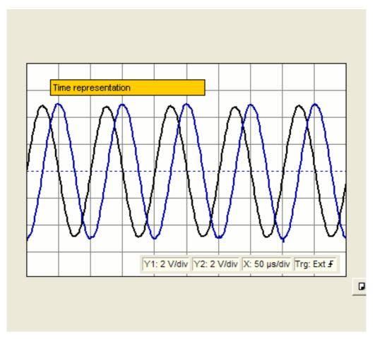
The oscillograms show clearly in the time representation the phase shift of -90° between the two carrier signals in the upper and lower 2PSK branch of the 4PSK modulator. In the XY representation there is (depending on the scaling) an ellipse or (if the axes have the identical scale) a circle, since the carrier signals each represent a sinusoidal resp. cosinusoidal function.
