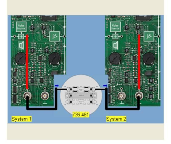
In the following experiment we will investigate simplex operation of two COM3LAB Master Units with the 700 74 Modem Technology experimenting board for sending over a transformer coupled twisted quad in baseband. Any desired texts are sent; transmission takes place without error checking and correction ('Parity' - none).
