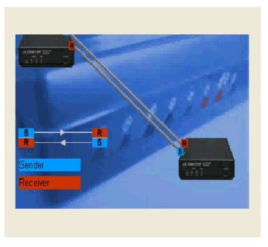
In full-duplex mode, or simply duplex<sup>1</sup> for short data can be sent simultaneously in both directions, in other words the respective devices function as both sender and receiver at the same time. Telephones and most modems use full-duplex connections. To use duplex mode over a single line, corresponding measures are required such as direction separation using a hybrid terminating circuit as used in telephones or a time or frequency multiplexing procedure.
