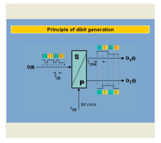
The digit signals  $D_1(t)$  and  $D_2(t)$  obtained by means of a serial-parallel conversion from the original bit sequence D(t). In principle this is an extension of the bit to the duration  $T_{Dibit} = 2T_{Bit}$  and a division into two separate signal sequences. The first bit in a bit pair is delayed by the time duration of one bit in order to bring both dibit signals to the same clock start.
