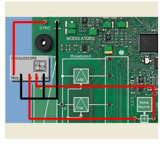
In the following experiment we will analyze the noise signal in the time and frequency ranges. A squarewave signal which is sent in the baseband will be additively overlaid. Note that the COM3LAB noise generator can, for didactic purposes, generate significantly higher error rates than actually occur in commercial systems!
