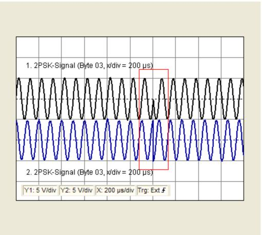
The oscillograms show clearly the phase shift of -90° between the two carrier signals in the upper and lower 2PSK branch of the 4PSK modulator. Since both branches perform "normal" 2PSK modulation, the result for 0-1- and 1-0- edges of the data signal are jumps of 180° each.
