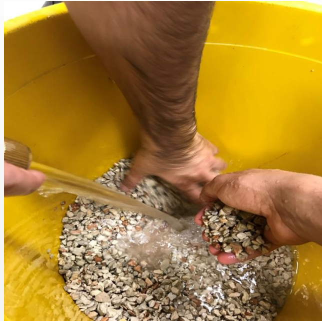
Washing of Aggregate
