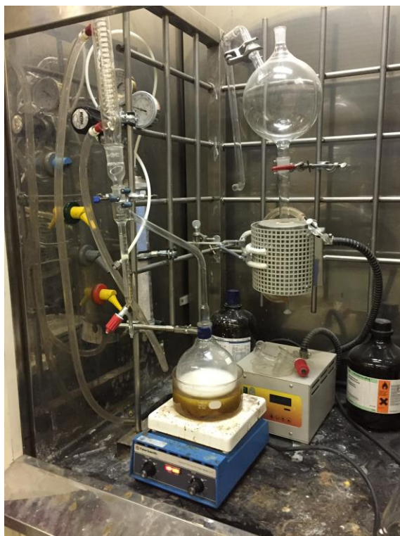
Figure 1: Preparation of mono basic sodiumphosphate using Dean-Satrk apparatus
